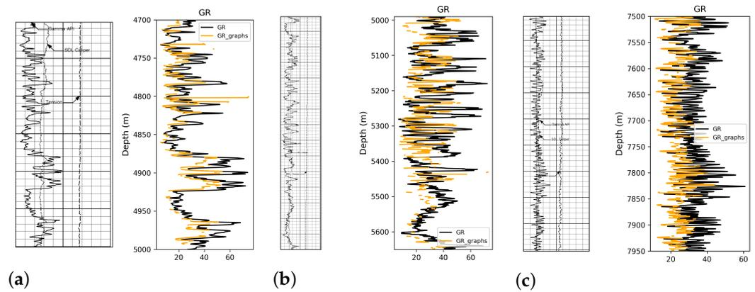
**Figure 7.** Comparison between native LAS Gamma Ray and the graph-based method with corresponding depth sections of the raster log image. (a) Depth 4700 to 5000 m; (b) Depth 4990 to 5650 m; (c) 7500 to 7950 m.
