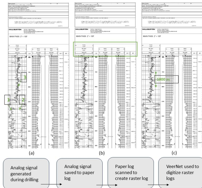
**Figure 1.** (a) 1,2,3 logs corresponding to GR, Caliper, and tension. (b) Header section showing the scales, of curves (c) depth line coding for 5'' log corresponding to 1000 m. Bottom: Flow chart showing the proposed approach.
