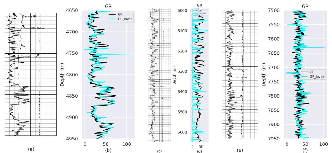
**Figure 3.** Comparison between the ground truth and prediction from the model trained using Lovasz Loss. (a) Rsater Log-Depth 4700 to 5000 m; (c) Rsater Log-Depth 4990 to 5650 m; (e) Rsater Log-Depth 7500 to 7950 m. (b,d,f) represent the fit between Ground Truth (GT) and predicted GR values for (a–c), respectively.
