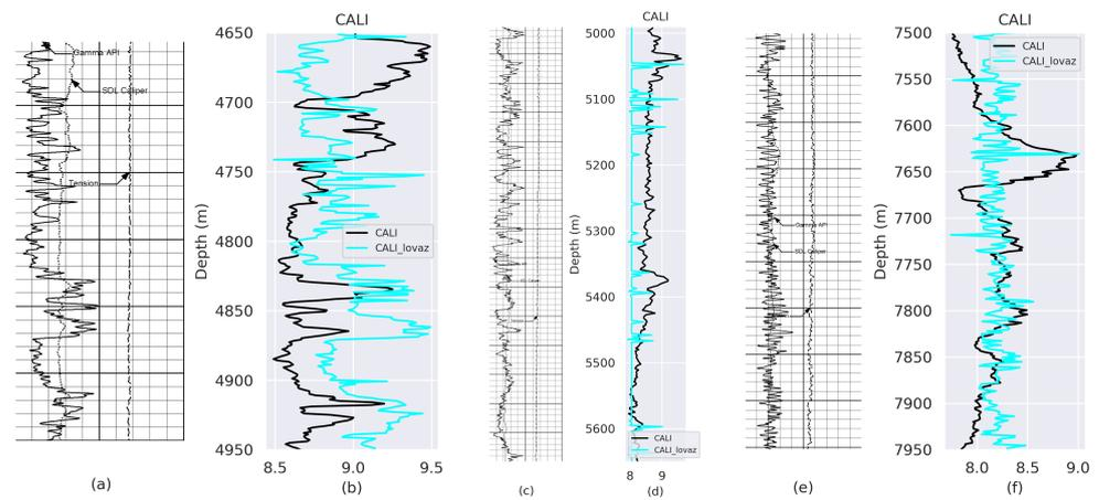
**Figure 6.** Comparison between GT and prediction from model trained using Lovaz Loss. (a) Rsater Log-Depth 4700 to 5000 m; (c) Rsater Log-Depth 4990 to 5650 m; (e) Rsater Log-Depth 7500 to 7950 m. (b,d,f) represent the fit between GT and predicted CALI values for (a-c), respectively.
