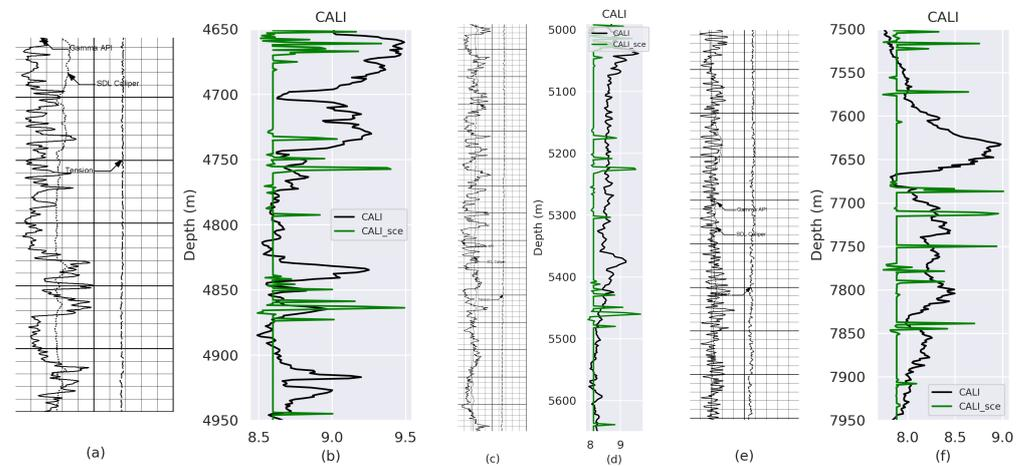
**Figure 5.** Comparison between GT and Prediction from model trained using SCE Loss. (a) Rsater Log-Depth 4700 to 5000 m; (c) Rsater Log-Depth 4990 to 5650 m; (e) Rsater Log-Depth 7500 to 7950 m. (b,d,f) represent the fit between GT and predicted CALI values for (a–c), respectively.
