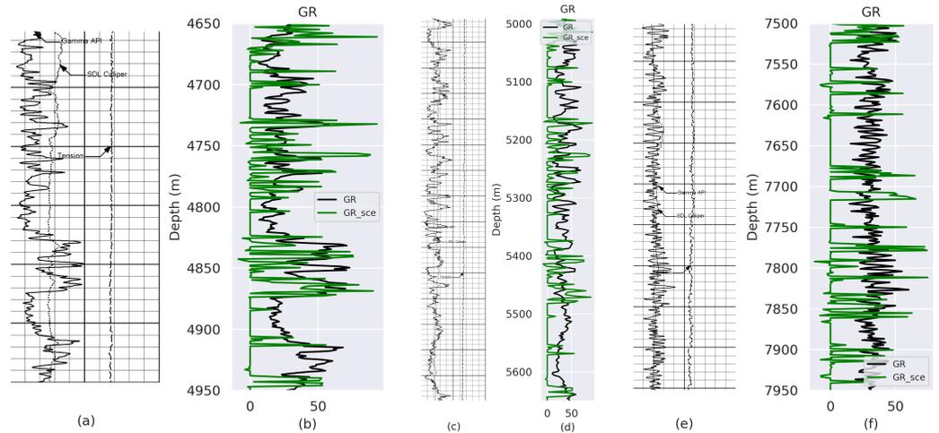
**Figure 4.** Comparison between GT and prediction from model trained using SCE Loss. (a) Rsater Log-Depth 4700 to 5000 m; (c) Rsater Log-Depth 4990 to 5650 m; (e) Rsater Log-Depth 7500 to 7950 m. (b,d,f) represent the fit between GT and predicted GR values for (a–c), respectively.
