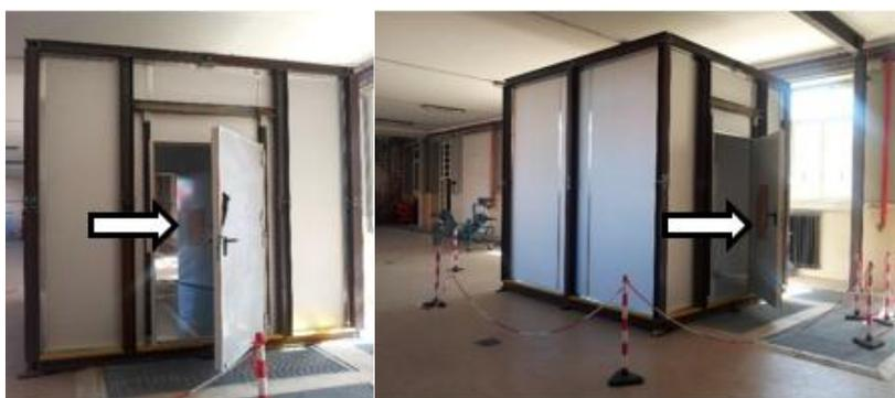
**Figure 3.** Experimental smokeproof enclosure (front and back door opening, respectively inwards and outwards).
