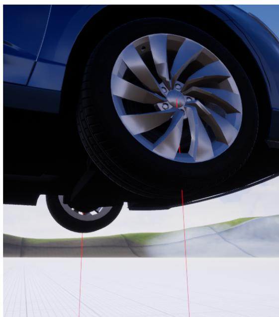
**Figure 4.** Wheels raycast curb detection.
