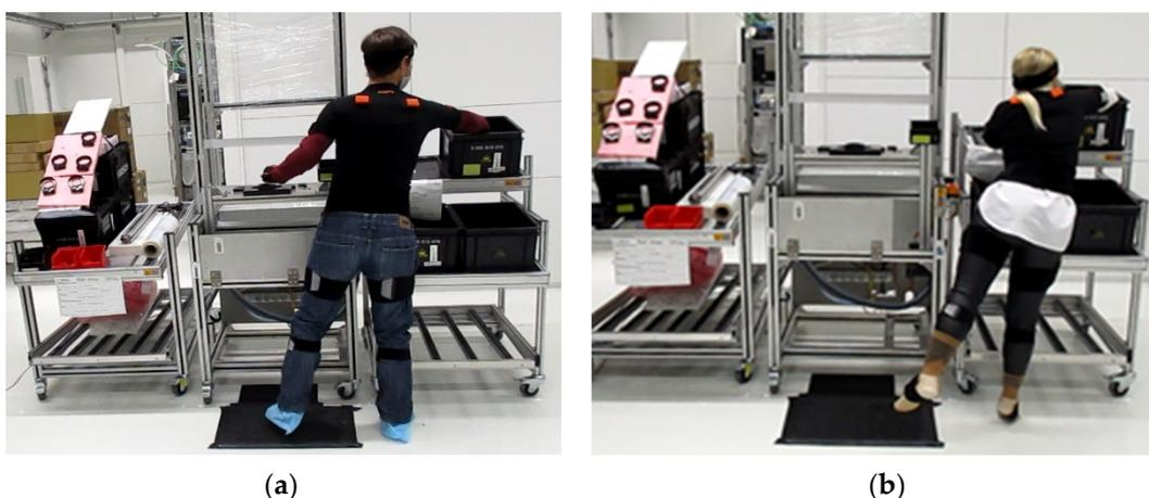
Figure 8. Assembly task with sensors for obtaining RULA scores: (a) Highest percentile; (b) Lowest percentile.
