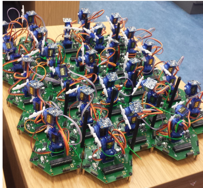
Figure 6. Multiple-tiled hexagonal cilia connected to each neighbour, sharing power and data.
