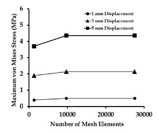
**Figure 9.** Maximum von Mises stress induced due to three different displacements applied on finite element meshes with a different number of elements, as part of the mesh convergence study.
