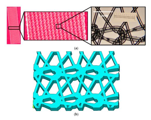
**Figure 4.** Two steps for prosthetic mesh model development. (**a**) Microscope images of the Prolene<sup>®</sup> prosthetic mesh showing the repetitive unit. (**b**) Simplified geometric model of the prosthetic mesh.
