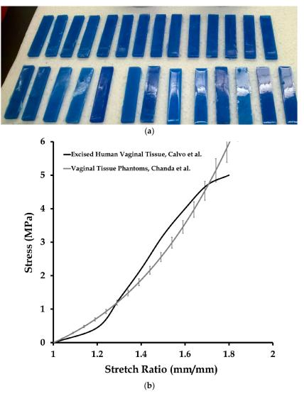
**Figure 2.** Mechanical testing of vaginal tissue phantoms. (**a**) Vaginal tissue samples. (**b**) Average and standard deviation of stress vs. stretch responses of 27 vaginal tissue phantoms tested by Chanda et al. [13–15], compared with average biomechanical properties of excised human vaginal tissue, tested by Calvo et al. [22]. Adapted from [22], Copyright 2009, with permissions from Elsevier. The strain rate for all the experiments was 0.08 mm/s.
