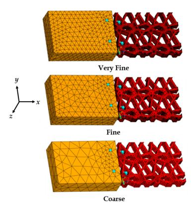
**Figure 5.** Finite element meshes of the vaginal tissue phantom, prosthetic mesh, and sutures, modeled for the mesh convergence study.
