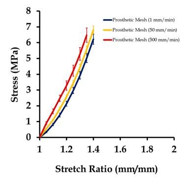
**Figure 7.** Stress vs. stretch plot of 15 prosthetic mesh samples tested under uniaxial loading (five samples each at 1, 50, and 500 mm/s). Data are shown as mean  $\pm$  standard deviation.
