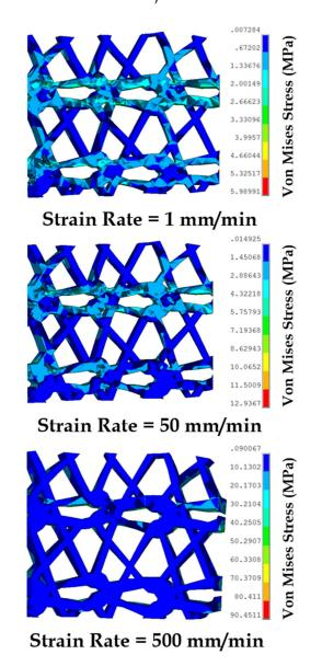
**Figure 13.** Stress distribution in the prosthetic mesh sutured to the vaginal tissue phantom, observed at a stretch of 1.4 during uniaxial tension tests conducted at varying strain rates.
