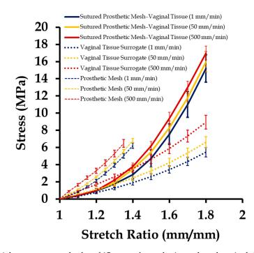
**Figure 8.** Uniaxial stress vs. stretch plot of 15 sutured prosthetic mesh and vaginal tissue phantom at strain rates of 1, 50, and 500 mm/min (five samples at each strain rate), compared with the stress–stretch responses of individually tested 12 vaginal tissue phantoms (four samples at each strain rate) and 15 prosthetic mesh (five samples at each strain rate). Data are shown as mean  $\pm$  standard deviation.
