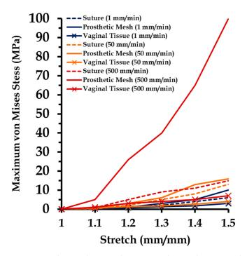
**Figure 12.** Maximum stresses at the prosthetic mesh, suture, and vaginal tissue panthom computational models stretched at different strain rates (1, 50, and 500 mm/min) in five load steps.
