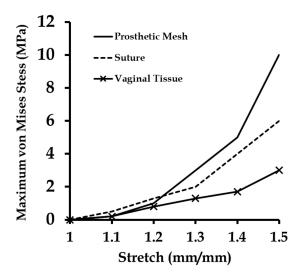
**Figure 11.** Maximum stresses induced at the prosthetic mesh, suture, and vaginal tissue phantom computational models as they were stretched together in uniaxial tension in five load steps (at a strain rate of 1 mm/min).
