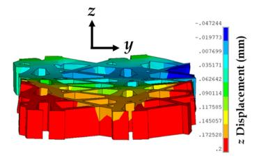
**Figure 14.** Representation of the prosthetic mesh showing a slight curling due to large and small *z*-displacements at the edges and mid-plane, respectively, for a tissue phantom–suture–mesh composite stretch of 1.4 and strain rate of 1 mm/min.
