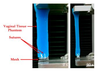
**Figure 3.** A uniaxial test conducted on a sutured prosthetic mesh and vaginal tissue phantom at 50 mm/min strain rate. Images taken at 0 and 90 s.
