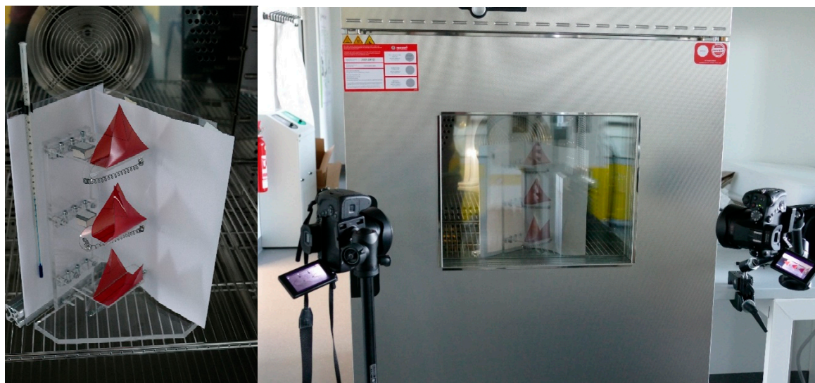
Figure S5. Climate chamber setup for SMA-spring demonstrator measurements. Three VFs with attached SMA springs were tested simultaneously (left). They were mounted on a plexiglass shelf and placed in a climate chamber (Memmert CTC 265) (right).
