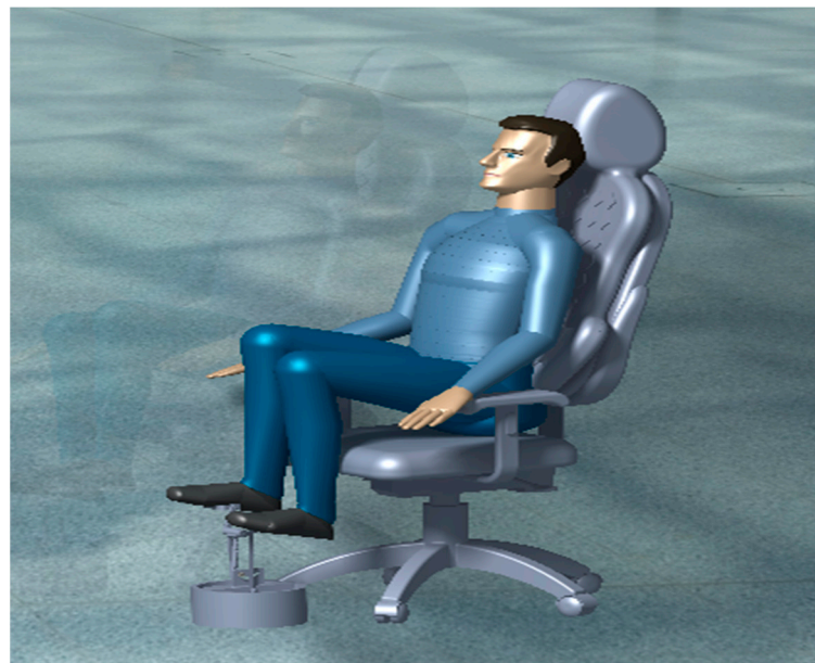
Figure 6. The manual blowing system with the pedaling mechanism.
