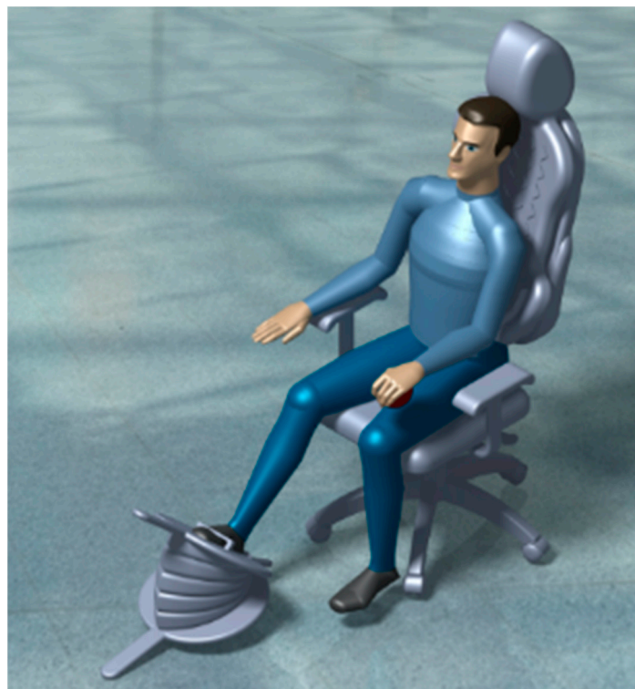
Figure 2. The seated person is using the accordion blower system.
