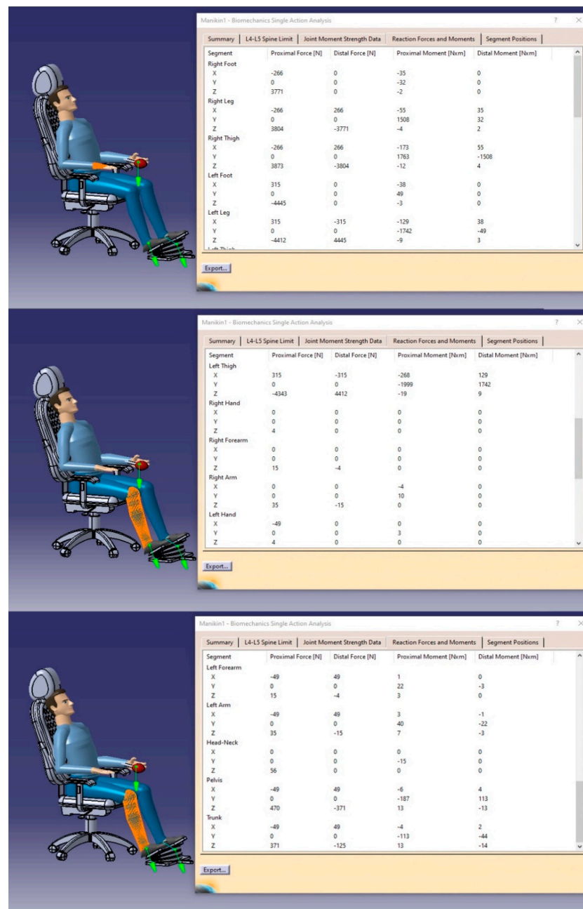
Figure 19. The data of the reaction forces and moments of the whole-body segments.
