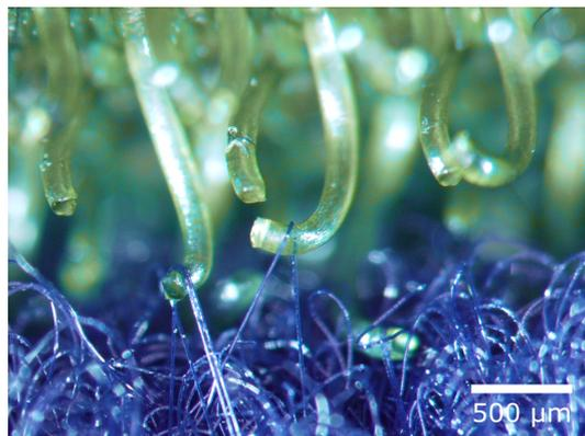
**Figure 14.** Hook-and-loop fastener (Velcro®) with hook tape (top) and loop tape (bottom).
