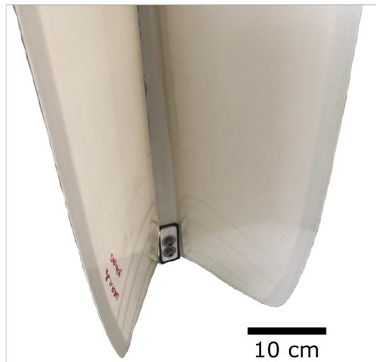
**Figure 20.** Detailed view of a demonstrator of the biomimetic Flectofin<sup>®</sup> facade shading system. The more the backbone is bent, the more the two lamellae fold sideways.
