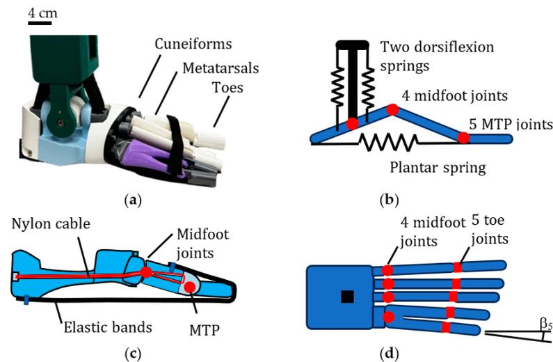
**Figure 6.** Bio-inspired foot design. (a) Prototype (no plantar fascia). (b) Schematic side view. (c) Section showing nylon cable (d) Plan view of foot.
