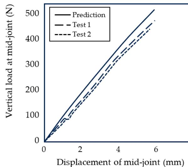
**Figure 9.** Vertical stiffness of the arch at the midfoot joint.
