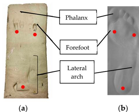
Figure 11. Contact patch of the bio-inspired foot and human foot (right foot). (a) Bioinspired foot (b) Human foot.
