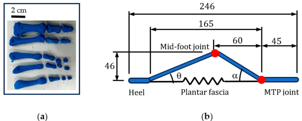
**Figure 5.** An adult female foot was used to determine key geometric points. (a) Three-dimensional printed bones (b) Geometry of middle toe.
