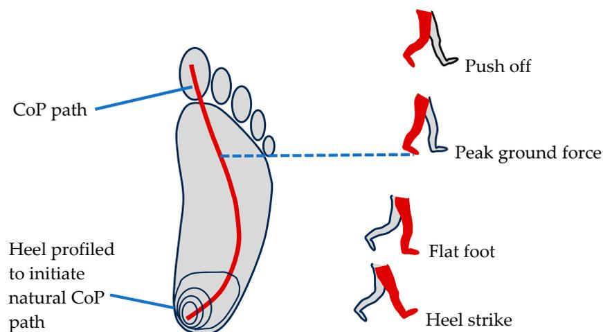
**Figure 12.** Profiled heel to initiate natural CoP pathway.
