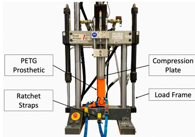
**Figure 8.** Stiffness test on the bio-inspired foot.
