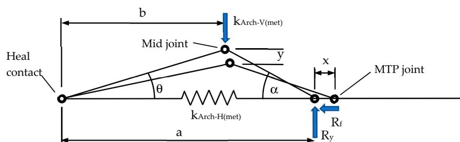
Figure 7. Model of each metatarsal arch as a mechanism.
