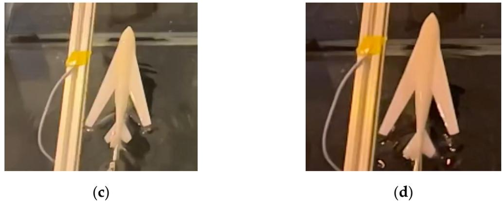
**Figure 34.** Waterbody response in the typical stage of slight water cross-over angle. (a) Close to the water surface; (b) the nose leaves the water; (c) the wing goes into the water; (d) the tail goes into the water.
