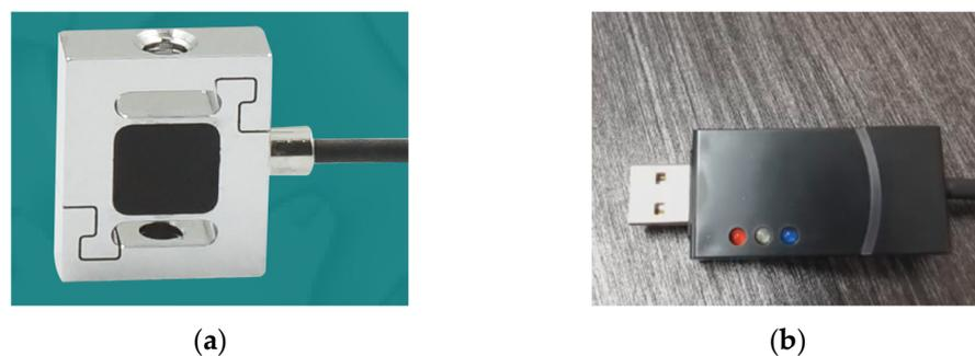
**Figure 32.** Sensor and data acquisition device. (a) AR-DN20 S-type tension and pressure sensor; (b) USB06 acquisition card.
