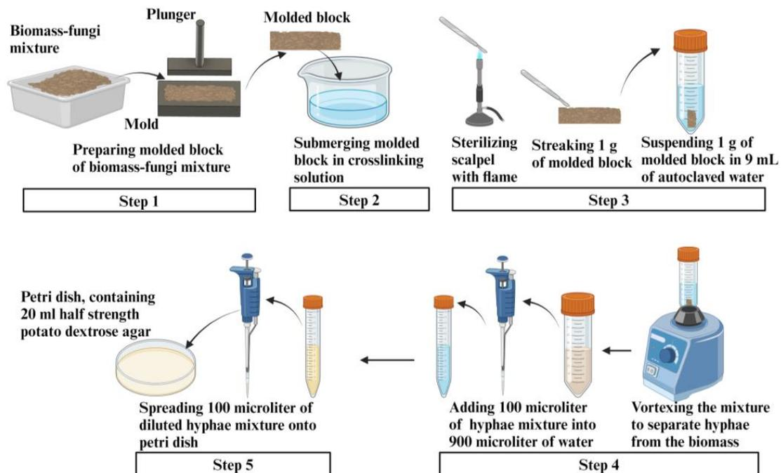
Figure 8. Preparing procedure for plated samples.
