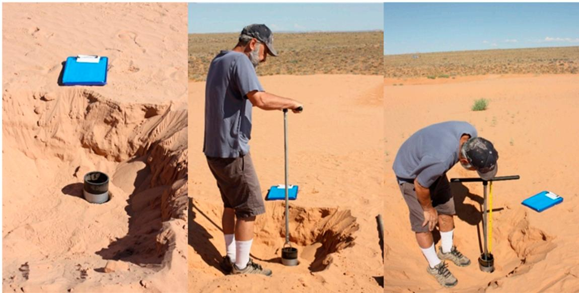
**Figure 1.** Hand-augering in Kanab Sand Dunes, southern Utah. Polyvinyl chloride (PVC) casing is inserted in top of auger hole to provide a reference platform for depth control and prevents influx of surface sediment downhole. The drill stem is advanced through the casing to the desired depth.
