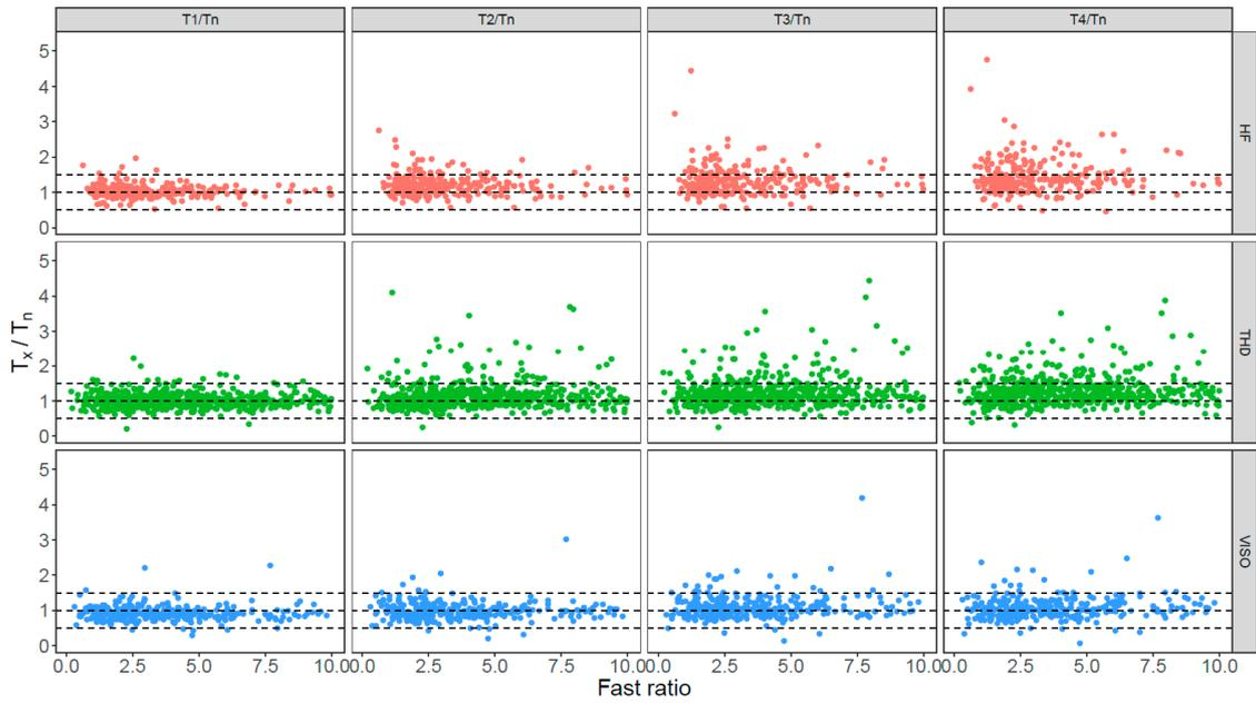
**Figure S1.** Ratios between test-dose signals ( $T_x$ ) of the 2<sup>nd</sup>–5<sup>th</sup> SAR cycles ( $T_1$ – $T_4$ ) and the first cycle ( $T_n$ ) plotted against fast ratio for grains from different sites (shown in different rows). The dashed horizontal lines represents values at 0.5, 1.0 and 1.5, respectively.
