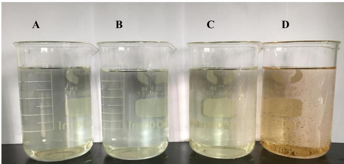
**Figure 1.** Chemical reaction result of Fe ion in normal seawater and *U. prolifera* degradation water environments. (A): normal seawater; (B): *U. prolifera* degradation water; (C): chemical reaction result of Fe ion in normal seawater; (D): chemical reaction result of Fe ion in *U. prolifera* degradation water.**Table 3.** Growth performance parameters and survival rate of the Japanese flounder cultivated in different environments.
