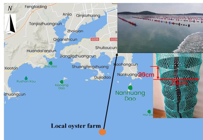
**Figure 1.** Location and image of the investigated longline aquaculture farm with lantern nets at a distance of 6.4 km from Nanhuang Island, Shandong Province, China, and the prototype of the lantern net with eight porous disks (material: rubber) with a diameter of 29 cm.
