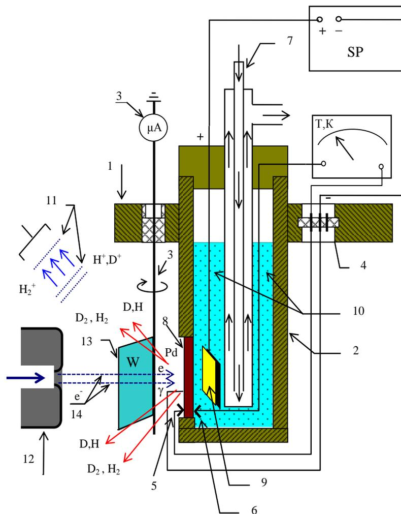
**Figure 5.** Cell for studying in situ processes of nonequilibrium migration of hydrogen and deuterium in metals: 1—flange; 2—a glass for electrolysis; 3—microammeter for measuring the electron beam current; 4—vacuum current leads; 5, 6—thermocouples; 7—flowing refrigerator; 8—test sample; 9—platinum electrode; 10—electrolyte; 11—mass spectrometer; 12—electron gun; 13—tungsten plate; 14—electron gun; and 15—the cell’s power supply.
