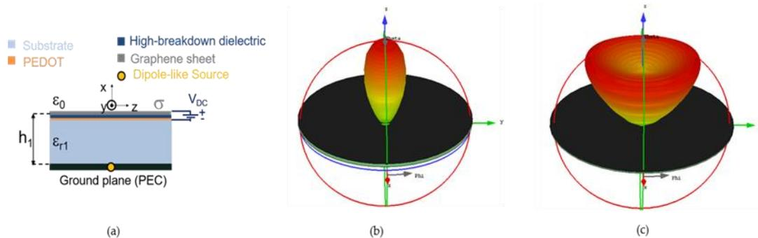
**Figure 6.** (a) a sketch of the GPW described in 5.1 [55]. In (b,c), the evolution from a pencil beam to a conical beam as the chemical potential is lowered from 1 eV to 0.5 eV, respectively [70]. The radiation patterns are obtained through CST full-wave simulations [58].
