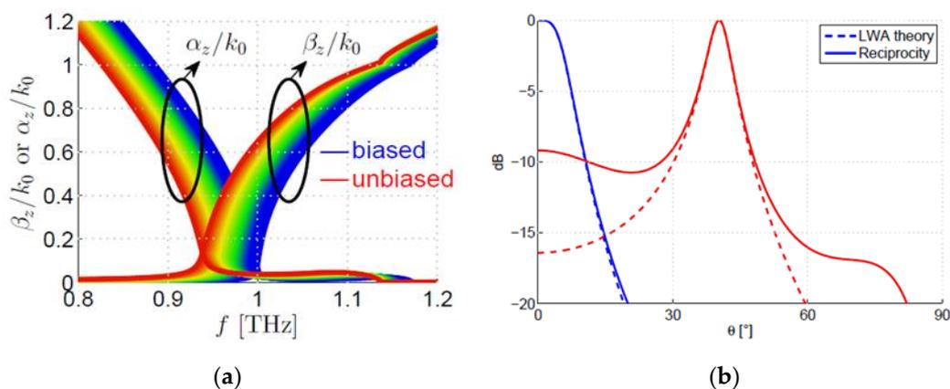
**Figure 3.** (a) dispersion curves of the fundamental TM mode computed by means of leaky-wave theory [55,56]; (b) radiation patterns predicted by leaky-wave theory (dashed lines) or by means of full-wave simulations with CST (solid lines) [55,56,58].
