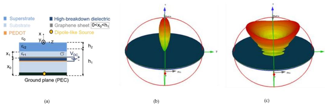
**Figure 7.** (a) a sketch of the GSS described in 5.2 [55]. In (b) and (c), the evolution from a pencil beam to a conical beam as the chemical potential is lowered from 1 eV to 0.3 eV, respectively [70]. The radiation patterns are obtained through CST full-wave simulations [58].
