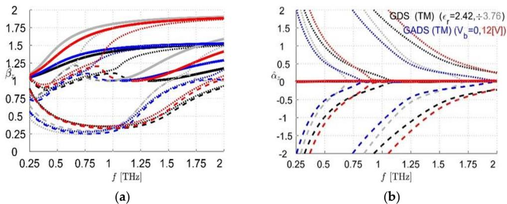
**Figure 5.** (a) normalized phase constant and (b) normalized attenuation constant spectra of the TM modes of a GDS (black and gray lines) and a GADS (red and blue lines) obtained by changing the values in the LC permittivity tensor. Proper modes are depicted in solid lines, physical and nonphysical improper complex modes are represented in dotted and dashed lines, respectively [59].
