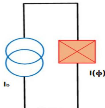
**Figure 1.** Schematic presentation of a phase qubit on the Josephson junction.
