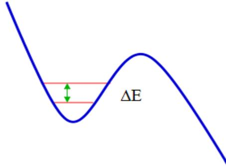
**Figure 2.** Profile of potential energy  $U(\phi) = -E_J \{\cos \phi + i_b \phi\}$  of the Josephson phase qubit.
