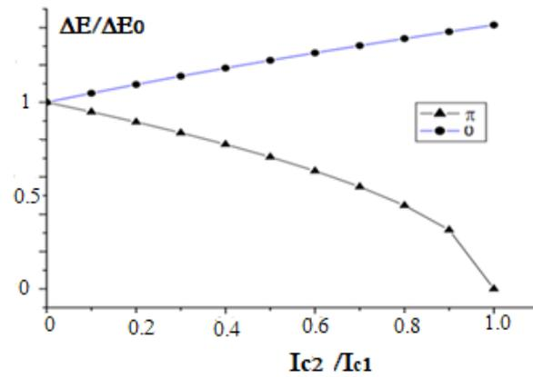
Figure 4. Changing the energy difference between levels  $\Delta E/\Delta E_0$  in qubit based on the single-/two-band junction versus  $I_{c2}/I_{c1}$ .
