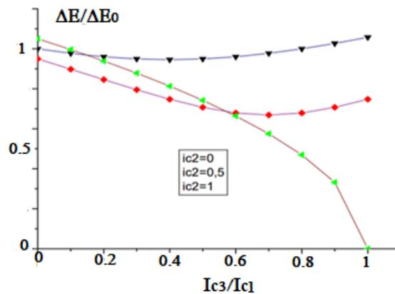
Figure 5. Changing the energy difference between levels in qubit based on single-/three-band junction  $\Delta E/\Delta E_0$  versus  $I_{c3}/I_{c1}$  for  $I_{c2}/I_{c1} = 0, 0.5, 1$  (from top to bottom).
