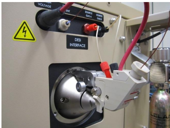
Figure S-2. Combination ESI/DESI source included with the FLIR AI-MS 1.2. ESI-MS is useful when examining extracts and dilute solution, while DESI-MS has proven is useful for the direct analysis of surfaces of simple geometry.
