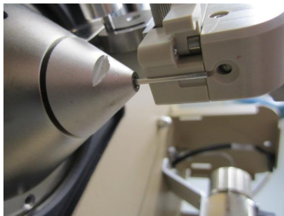
Figure S-3. Bottom-up view of the ESI/DESI emitter in relation to the inlet capillary of the AI-MS 1.2. The hemispherical enclosure allows placement of flat materials for sampling.
