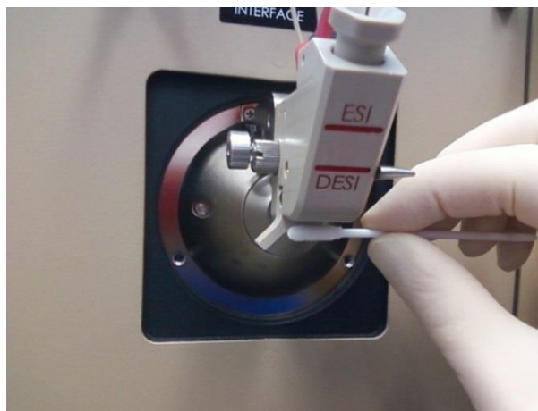
Figure S-5. DESI-MS analysis depicted directly from foam-based, surface-transfer swabs (Lab-Tips foam swab, Berkshire Corporation, Great Barrington, MA)
