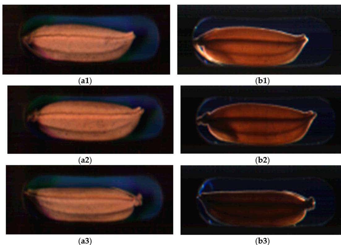
**Figure 6.** Pictures of the paddy rice kernels from the visual camera (a) and translucency camera using polarized light (b). The first kernel is a perfect kernel without dark areas. The bottom kernel is completely dark which indicates high chalkiness. The middle kernel has a local dark region, which indicates a chalky area close to the germ.
