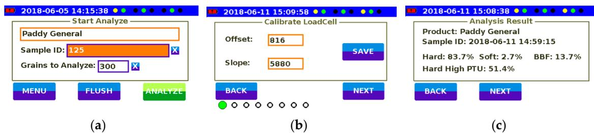
**Figure 2.** Touchscreen with selectable menus and displays. (a) Settings to define before analysis; (b) Settings to calibrate the load cell; (c) The results.
