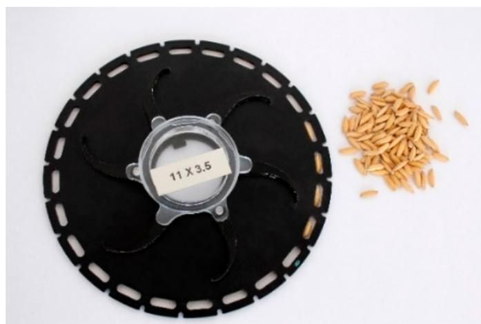
**Figure 3.** Singulation disc with cavity size of 11 × 3.5 mm.
