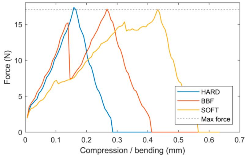
Figure 8. Example of texture measurement of a Hard kernel, a BBF kernel and a Soft kernel. The x-axis shows compression/bending deformation of the kernel and the y-axis shows the measured force. Note that the Hard kernel requires a high force for a small deformation, whereas the Soft kernel deforms much more before reaching the max force. The BBF kernel broke after 0.14 mm deformation.
