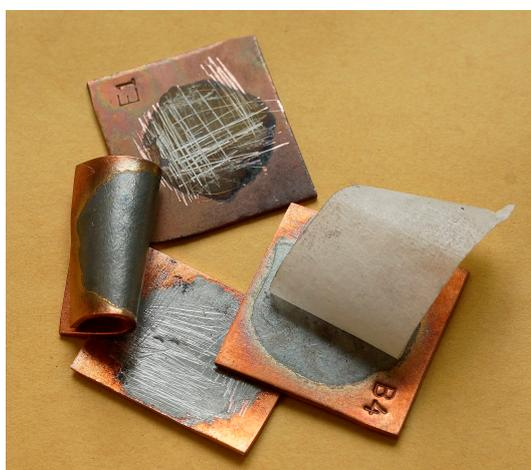
**Figure 4.** Tests for adhesion of coatings.
