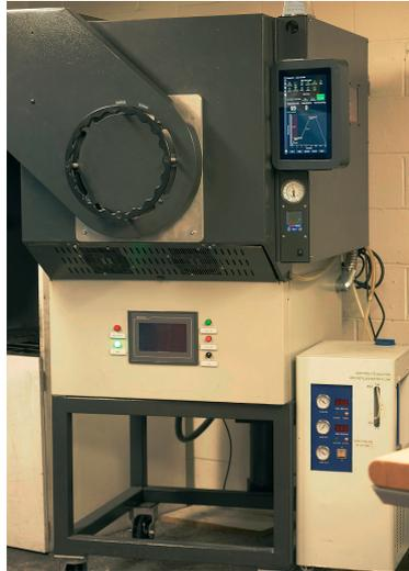
Figure 1. Hydrogen oven and H<sub>2</sub> generator.
