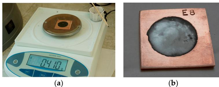
Figure 3. Application of the slurry: (a) Weighting the deposit (b) Sample coated, dried, and rolled.
