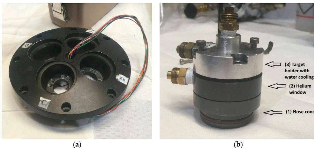
**Figure 1.** (a) TR13 four position target selector. (b) Standard TR13 solid target holder.
