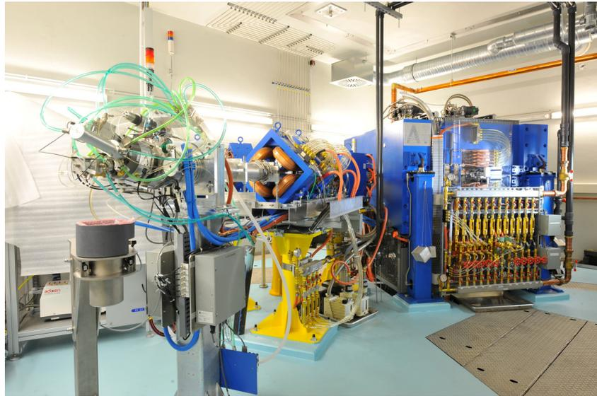
**Figure 3.** The TR-Flex cyclotron at the HZDR. The beamline 1B with a 4-port target selector is shown in the foreground. The second 4-port target selector is at the opposite side of the Cyclotron. Picture: HZDR/Frank Bierstedt.
