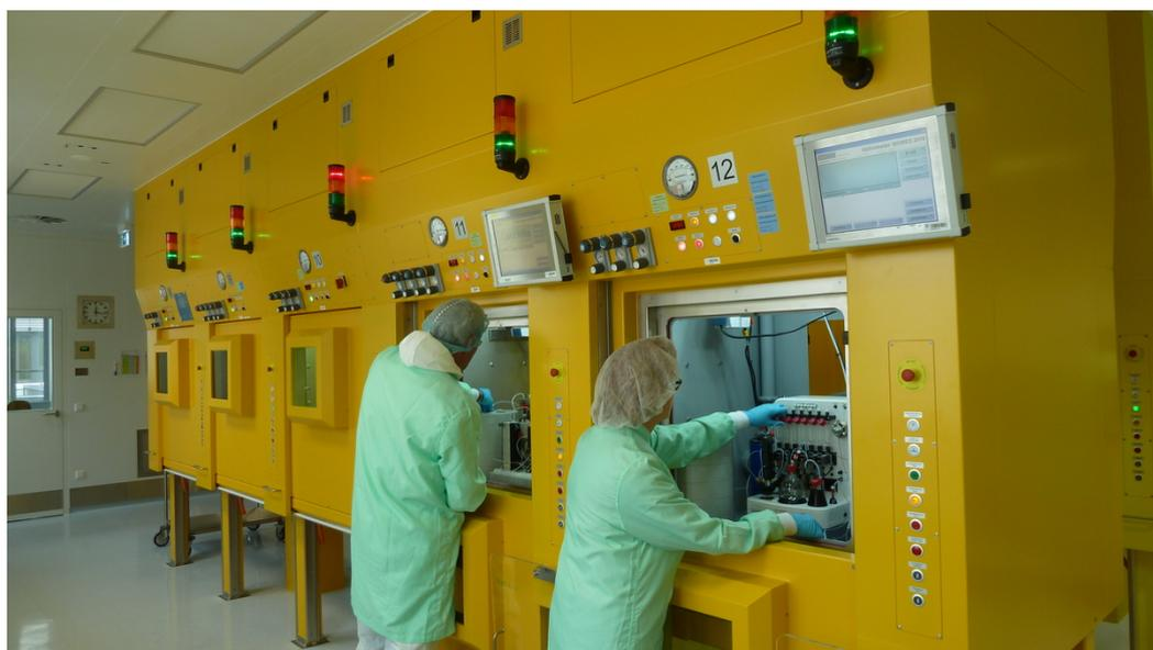
**Figure 2.** GMP area including the hot cells for the radiopharmaceutical production.
