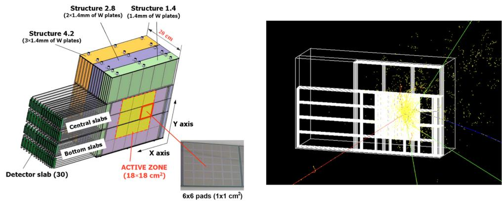
**Figure 6.** Left: Scheme of the CALICE SiW detector prototype from [17]. Right: Graphical representation of the Geant4 simulation of a  $\pi^-$  event interacting in the calorimeter via a nuclear inelastic process. See text for details.
