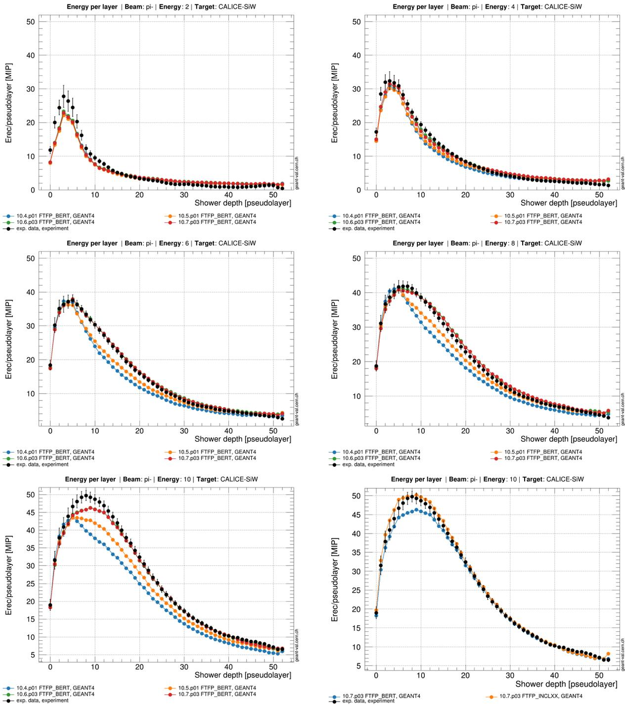
**Figure 7.** Longitudinal energy profiles for 2 (top-left), 4 (top-right), 6 (center-left), 8 (center-right), and 10 (bottom-left) GeV  $\pi^-$  events. Results from experimental measurements and Geant4 simulation with the FTFF\_BERT PL and releases from 2017 to 2020. **Bottom-right:** Comparison of the same variable as simulated with the FTFF\_BERT and the FTFF\_INCLXX PLs from the Geant4 10.7.p03 release.
