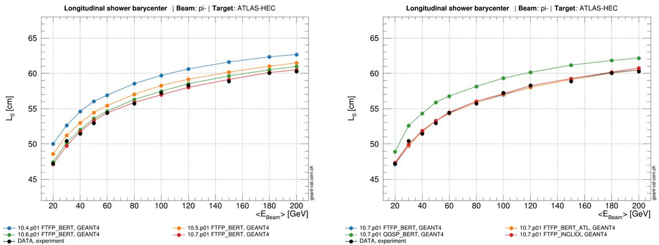
**Figure 4.** Left:  $L_0$  comparison of the Geant4 FTFP\_BERT PL prediction for recent releases (2017–2020) with the experimental data. Right: Comparison of several PL predictions from Geant4 10.7.p01 for the same variable.
