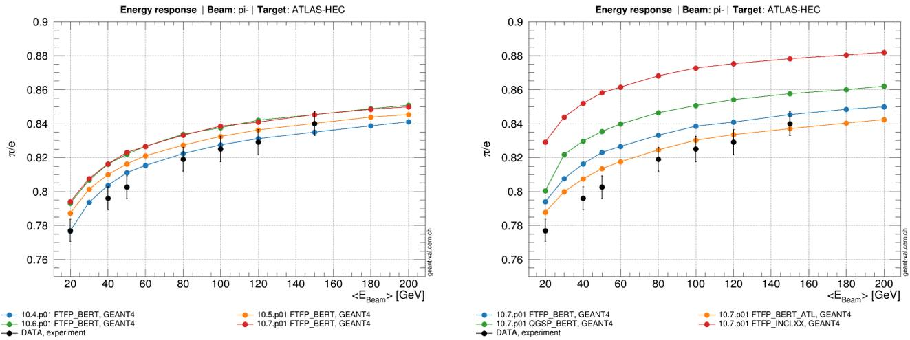
**Figure 2.** Left:  $\pi/e$  comparison of the Geant4 FTFP\_BERT PL prediction for recent releases (2017–2020) with the experimental data. Right: Comparison of several PL predictions from Geant4 10.7.p01 for the same variable.
