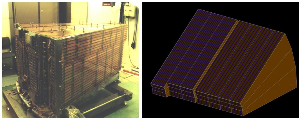
**Figure 1.** **Left:** Picture of three  $\phi$ -modules from a section of the ATLAS HEC first wheel from [13]. **Right:** Graphical representation of the three  $\phi$ -modules from a section of the ATLAS HEC, as simulated with Geant4.
