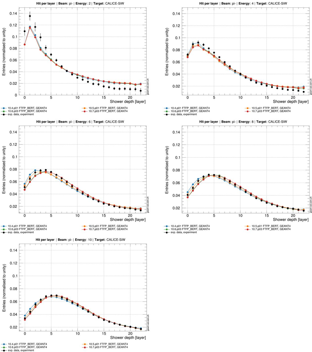
Figure 8. Longitudinal hit profiles for 2 (top-left), 4 (top-right), 6 (center-left), 8 (center-right), and 10 (bottom-left) GeV  $\pi^-$  events. Results from experimental measurements and Geant4 simulation with the FTFP\_BERT PL and releases from 2017 to 2020.
