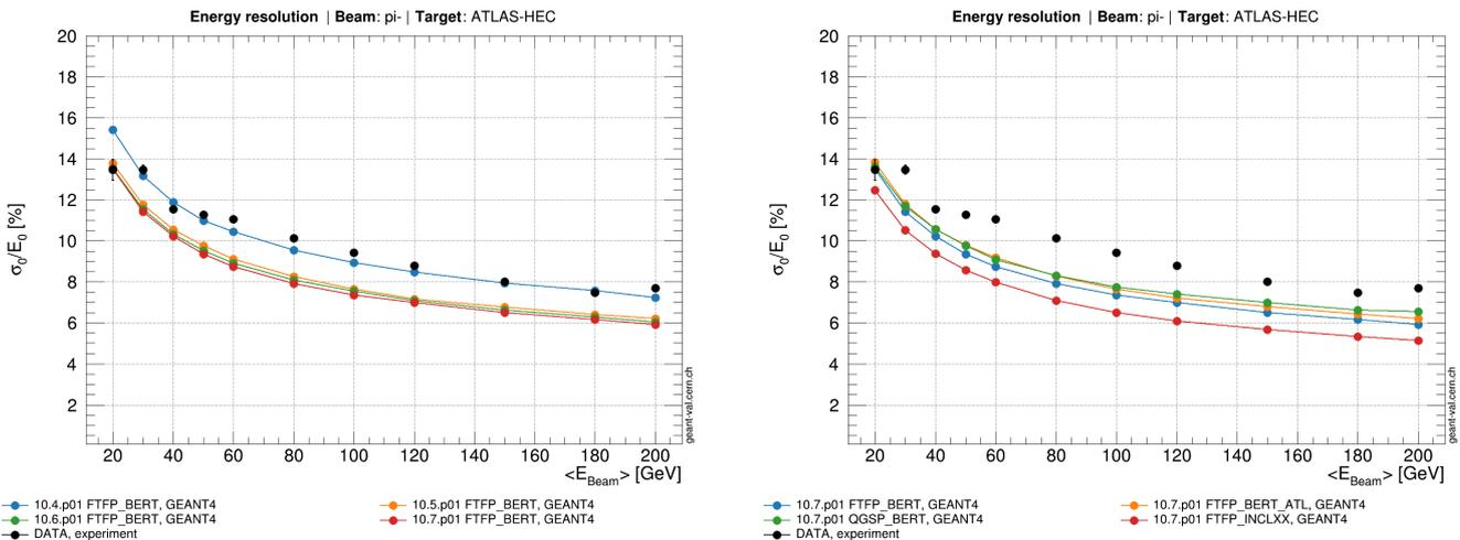
**Figure 3.** Left:  $\sigma/E$  comparison of the Geant4 FTFP\_BERT PL prediction for recent releases (2017–2020) with the experimental data. Right: Comparison of several PL predictions from Geant4 10.7.p01 for the same variable.
