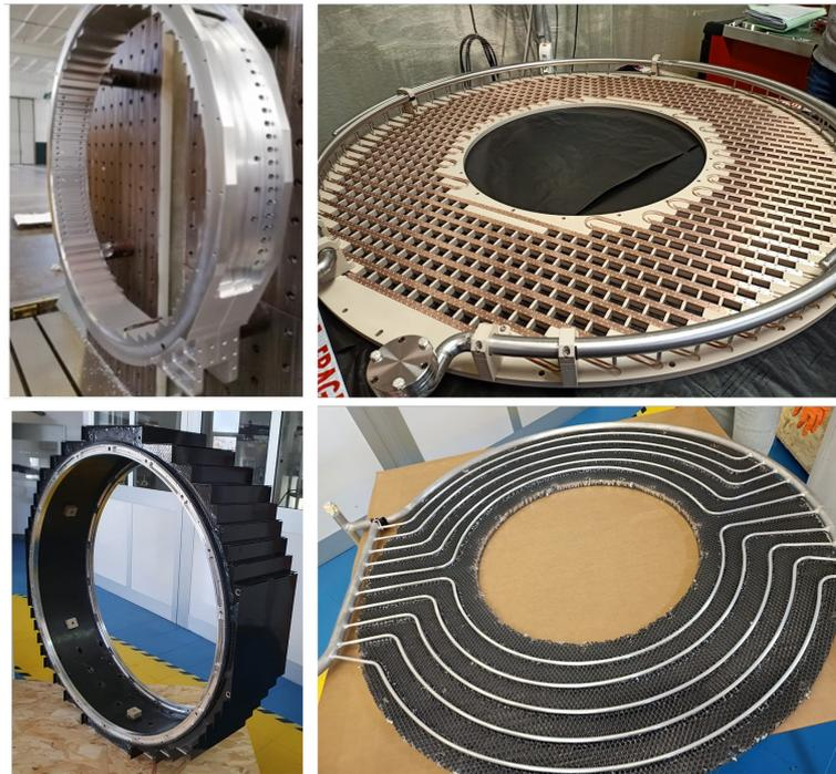
**Figure 6.** Calorimeter mechanical parts: (top left), outer ring; (top right), FEE plate; (bottom left), inner ring; (bottom right), front plate with source tubing embedded in the aluminium honeycomb.
