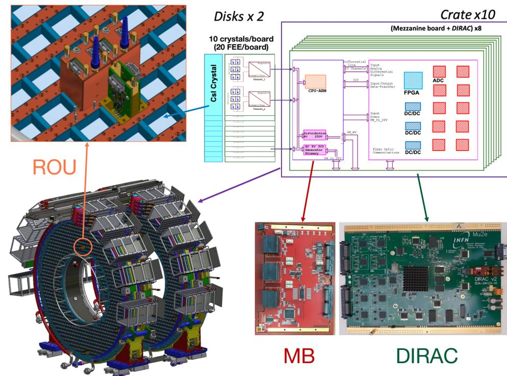
**Figure 1.** Overview of the Mu2e calorimeter readout system. Top-left: detail of the readout units (ROU) assembly in the calorimeter disk (heat exchangers are also visible). The electronics crates' architecture, including mezzanine (MB) and DiRAC boards, is also shown on the right.
