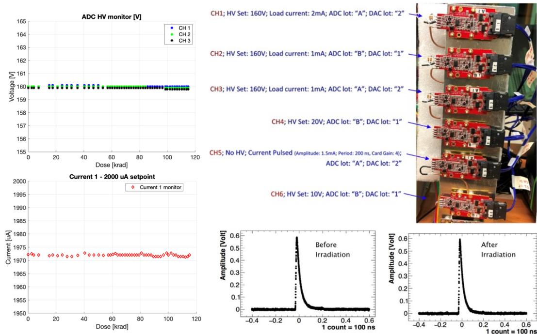
**Figure 8.** Top-right: configuration for the final FEE TID test. Left: example of stability plots for regulator voltage and current during irradiation. Bottom-right: waveforms comparison before and after TID irradiation.
