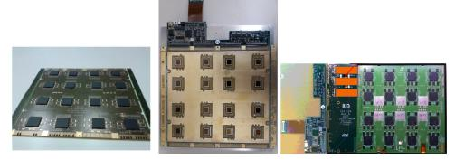
**Figure 5.** PCB variants that were used in the 2021 and 2022 beam tests. In the left and right ones, the ASIC are embedded in BGA packages. They differ by internal routing and external connectivity. The middle one features wire-bonded ASICs in cavities that are sunk into the PCB surface. The ASICS are protected by a transparent potting agent.
