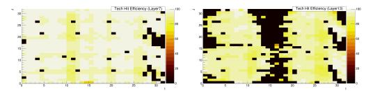
**Figure 9. Left:** Example for a layer with nearly complete acceptance. **Right:** Example for a layer with reduced acceptance mainly due to inefficiencies in the response to energy depositions. Here, *I*, *J* indicate the pad index and the color code represents the efficiency of a pad to energy depositions by MIP-like particles.
