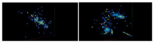
**Figure 10. Left:** A 20 GeV electron recorded in the SiW ECAL. **Right:** Two 20 GeV electrons in the SiW ECAL. The distance between the two showers is about 5 cm.
