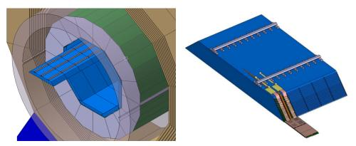
**Figure 2. Left:** A CAD drawing showing the electromagnetic calorimeter of ILD in light blue. The drawing is taken from [20]. **Right:** Drawing of an alveolar structure of a barrel module. The insertion of the slabs into the alveoli is indicated.
