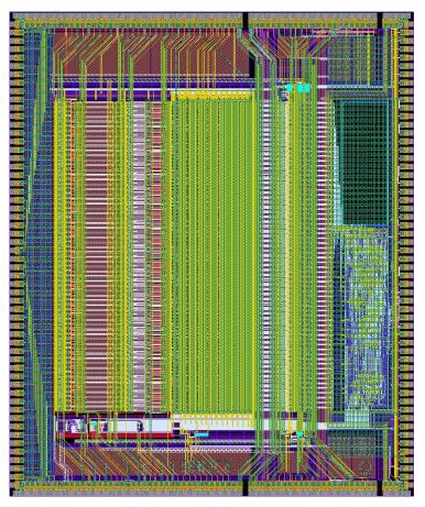
Figure 4. Image of the SKIROC2a front-end ASIC.
