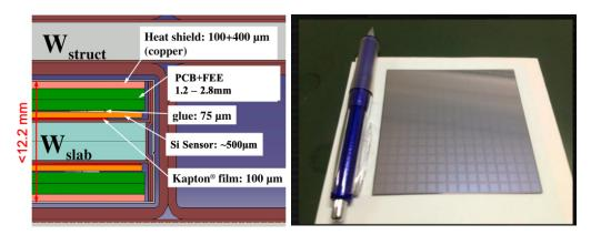
**Figure 3. Left:** Cross-section through a SiW ECAL slab. **Right:** Si sensor, the pads of size  $5.5 \times 5.5$  mm<sup>2</sup> are well visible.
