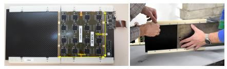
**Figure 7. Left:** Photo of a layer as used for the beam tests described in this article. Visible is the ASU, the SL-Board and the rails that hold in place ASU and tungsten absorber plates. **Right:** Photo of the insertion of the tungsten absorber plates.
