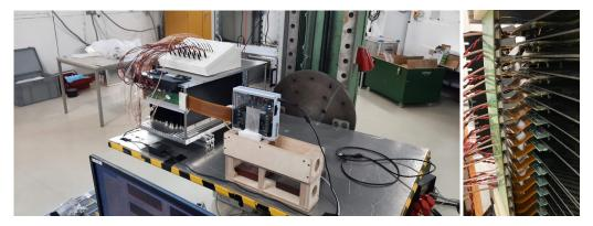
**Figure 8. Left:** Photo of the 15-layer stack of the CALICE SiW ECAL in the beam test area at DESY. Visible are the mechanical housing of the HV and LV cabling that supplies the 15360 cells of the stack as well as the flat kapton cable for data transmission and the CORE-Module. **Right:** Zoom into the extremities of the stack to appreciate the compactness of the ensemble.
