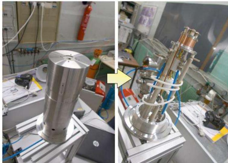
**Figure 3.** The final assembly of the ECR system.
