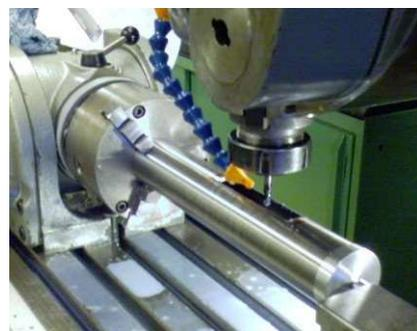
**Figure 6.** Photograph of the manufacturing of movable electrode of the Einzel lens.
