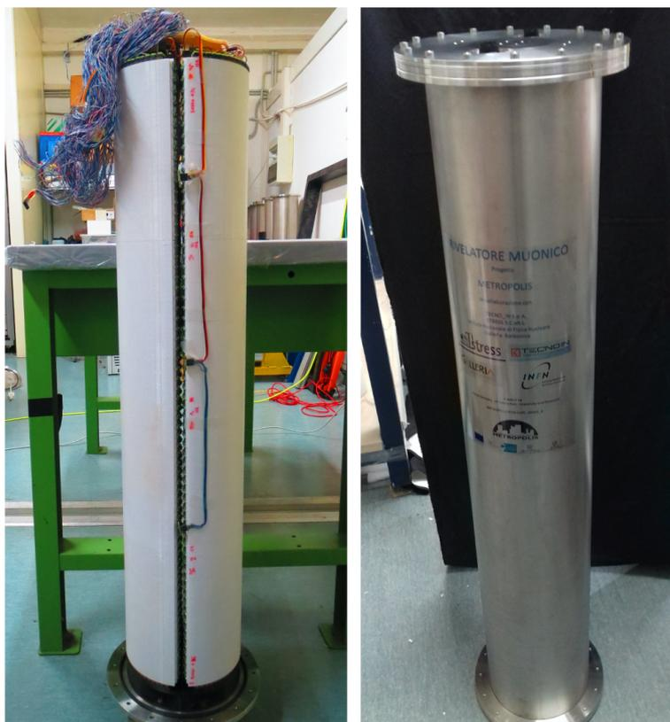
**Figure 3.** Final assembly of the cylindrical muon detector. On the left, the detector sensitive body before being inserted in the watertight shell (right).
