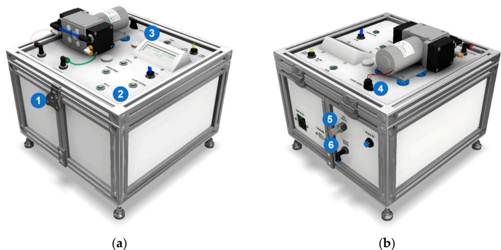
**Figure 5.** Computer model of the Testbed. (a) The front quarter view shows (1) the quick-turn draw latch, (2) the control panel, and (3) the custom LCD bezel. (b) The rear quarter view shows (4) the power plug for the pump, (5) the muffer for the gas exhaust, and (6) an elbow fitting pointing downwards to drain exhaust liquids.
