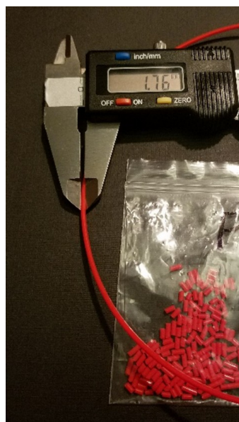
Figure 16. Example filament with a diameter of 1.75 \text{ mm} \pm 0.10 \text{ mm} made from RepRapable recyclebot, using the pelletized filament shown in the bag.
