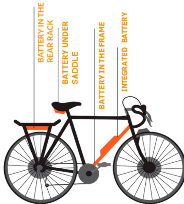
Figure 6. Types of battery layout.
