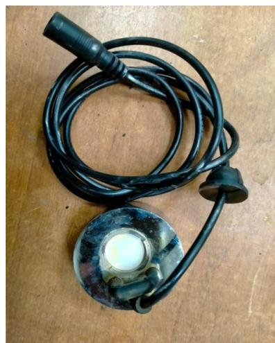
**Figure 4.** Ultrasonic humidifier.
