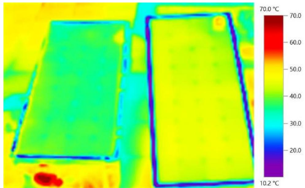
**Figure 8.** Thermal image for both panels, cooled (**left**) referenced (**right**).
