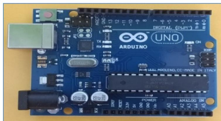
**Figure 10.** Arduino UNO implementation board.
