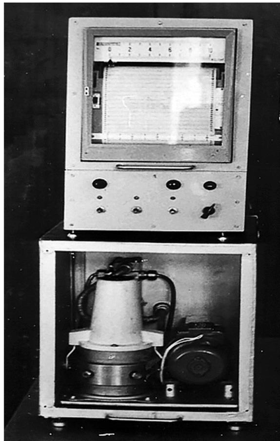
**Figure 12.** Automatic analyzer with tracking astatic balancing with the range of kinematic viscosity measurement  $(1-5) \cdot 10^{-6} \text{ m}^2/\text{s}$ .
