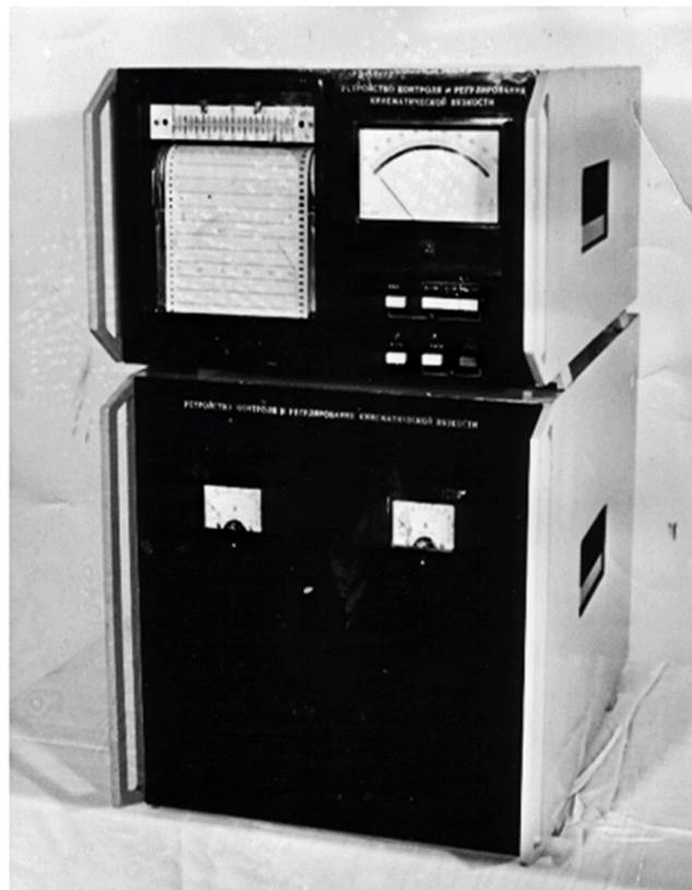
**Figure 13.** Automatic analyzer with tracking astatic balancing with the range of kinematic viscosity measurement  $(5-25) \cdot 10^{-6} \text{ m}^2/\text{s}$ .
