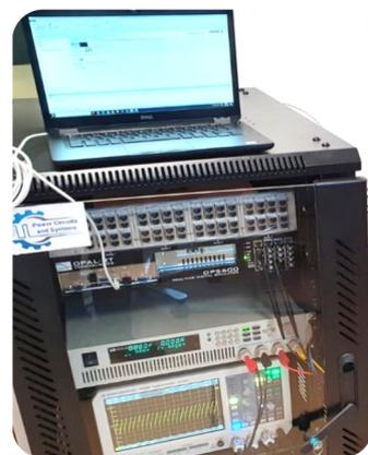
Figure 7. The Real-time setup of the SEFPC based on OPAL-RT.
