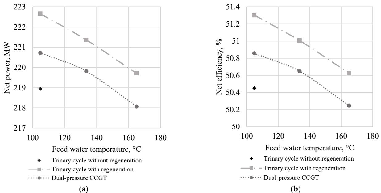
**Figure 17.** Net power and efficiency of trinary cycles at different feeding water temperatures: (a) net power, (b) net efficiency.
