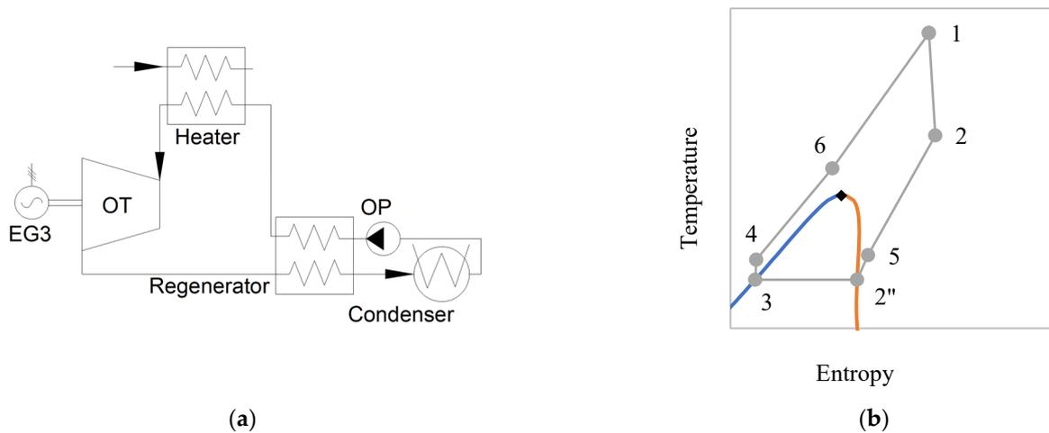
Figure 6. Organic Rankine cycle with regeneration: (a) plant, (b) supercritical cycle.
