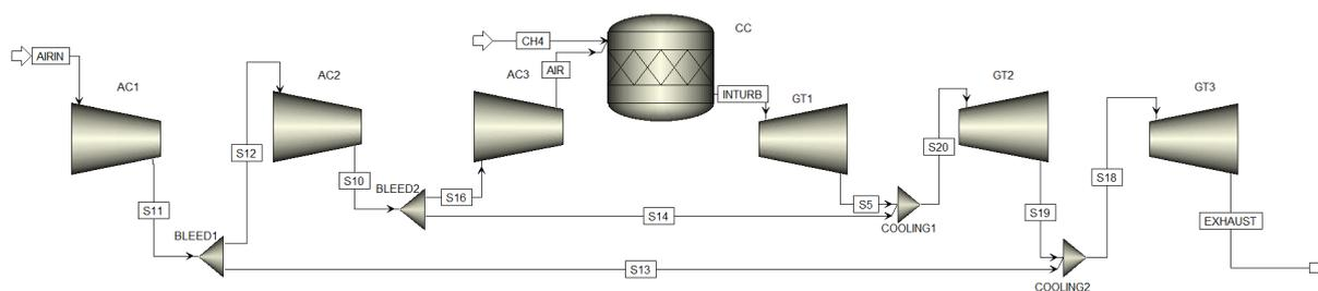
**Figure 8.** Cooled gas turbine model.
