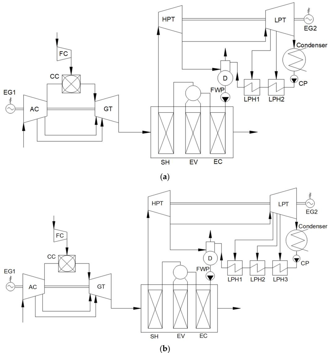
**Figure 3.** Single-pressure CCGT power plants with a cooled GT and a low-pressure regeneration system: (a) two LPHs, (b) three LPHs.
