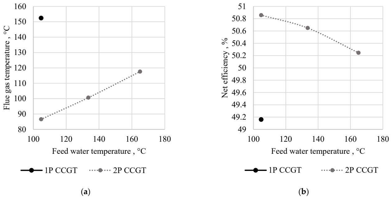
**Figure 14.** Dependence of the dual-pressure CCGT parameters on the feed water temperature: (a) flue gas temperature, (b) net efficiency.
