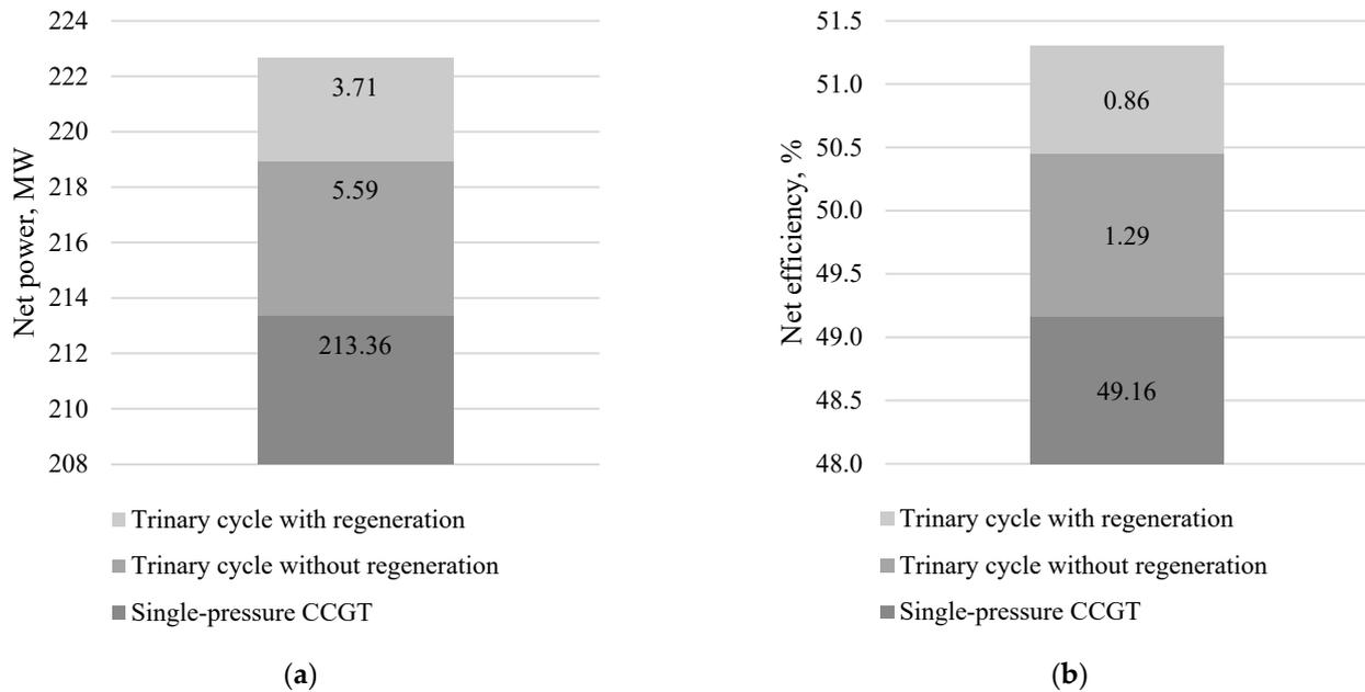
Figure 18. The effect of transition from single-pressure CCGT to trinary cycle: (a) net power, (b) net efficiency.
