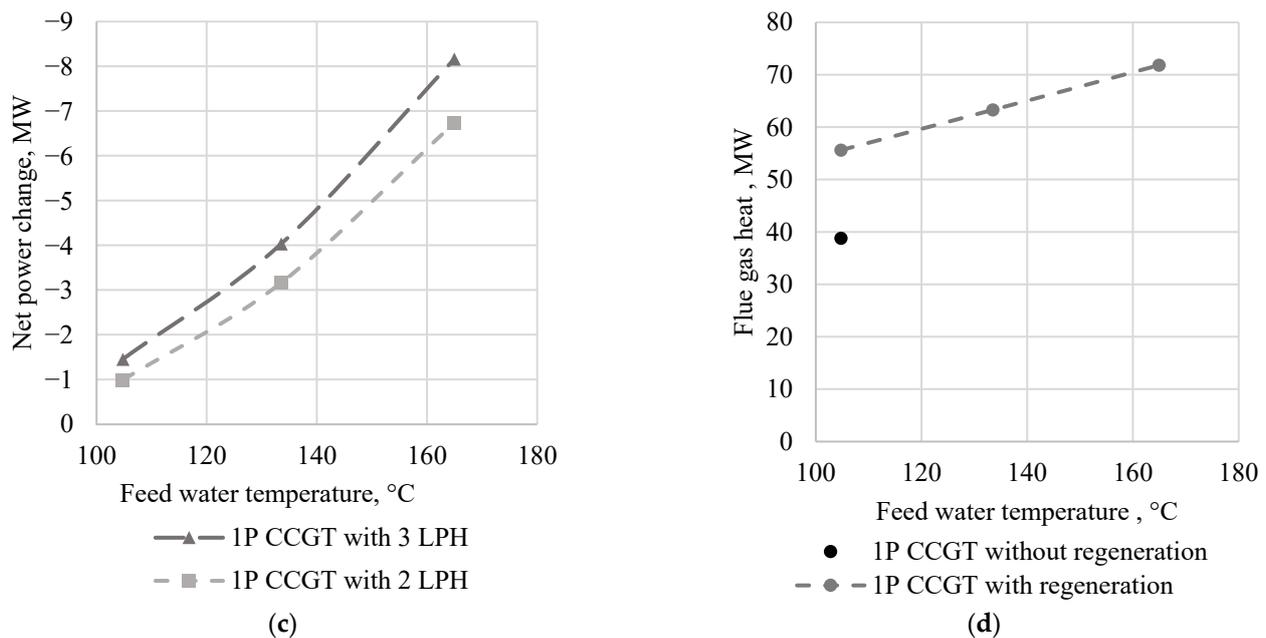
**Figure 15.** Influence of feed water temperature upon the CCGT characteristics: (a) the flue gas temperature, (b) net efficiency, (c) net power change, (d) flue gas heat potential when cooled to 80 °C.
