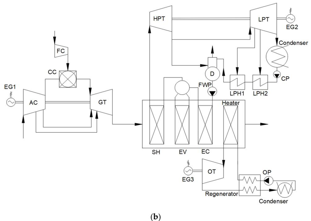
**Figure 7.** Trinary power cycles: (a) with a single-pressure CCGT, (b) with a single-pressure CCGT and low-pressure regeneration in STU.
