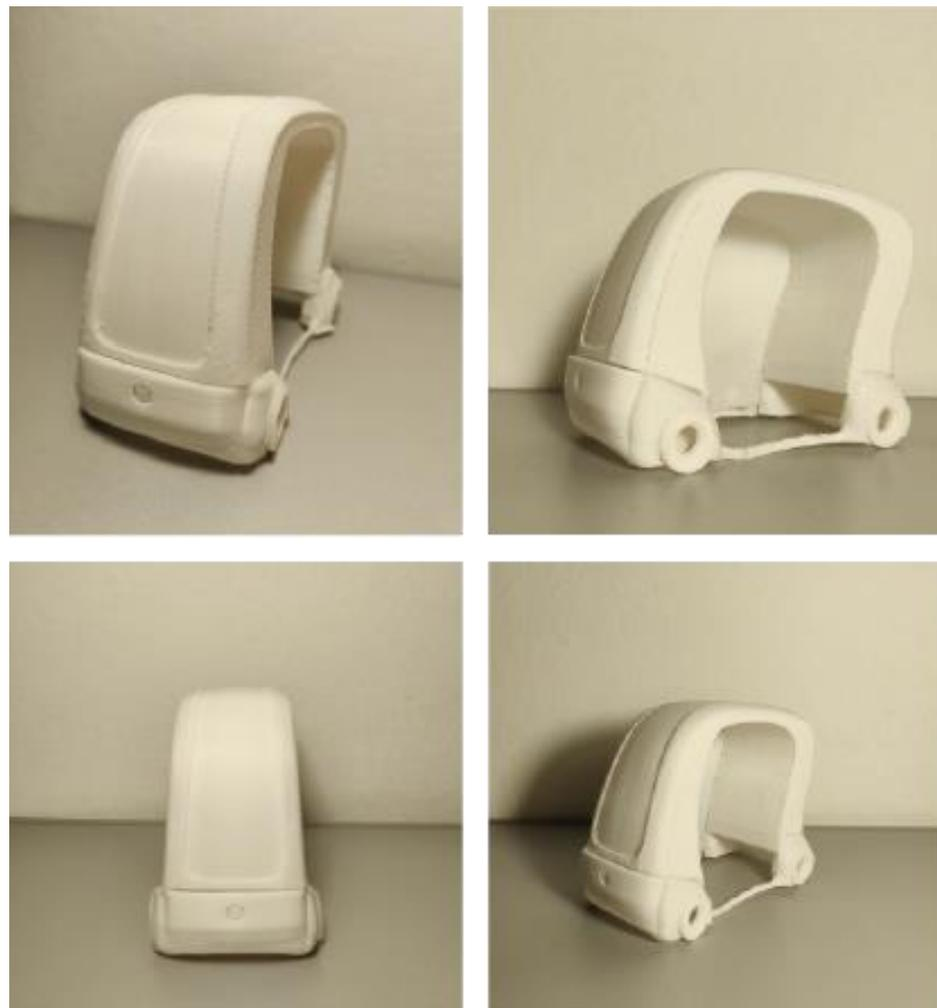
**Figure 28.** PLA 3D printed prototype of the final concept.
