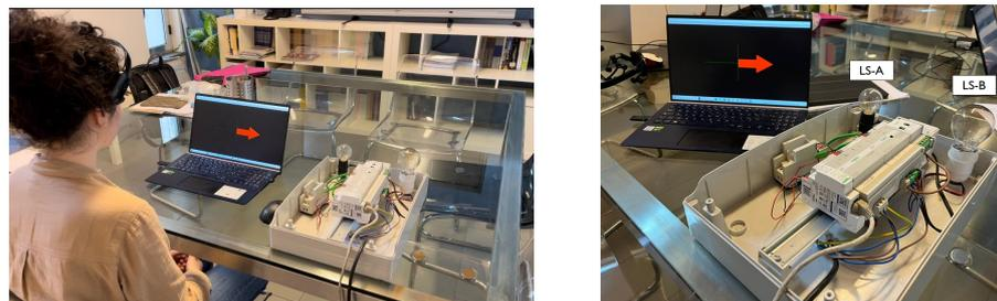
**Figure 1.** Experimental setup: a personal computer connected to two devices through KNX, i.e., two light bulbs.
