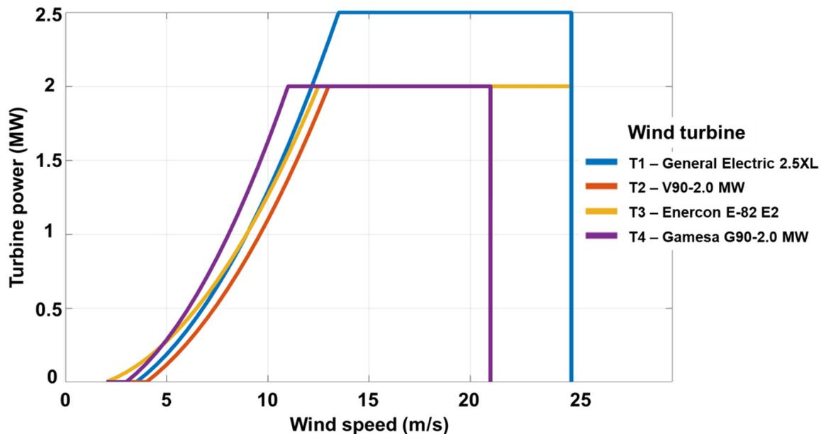
**Figure 2.** Power curves representation of the considered onshore wind turbines.
