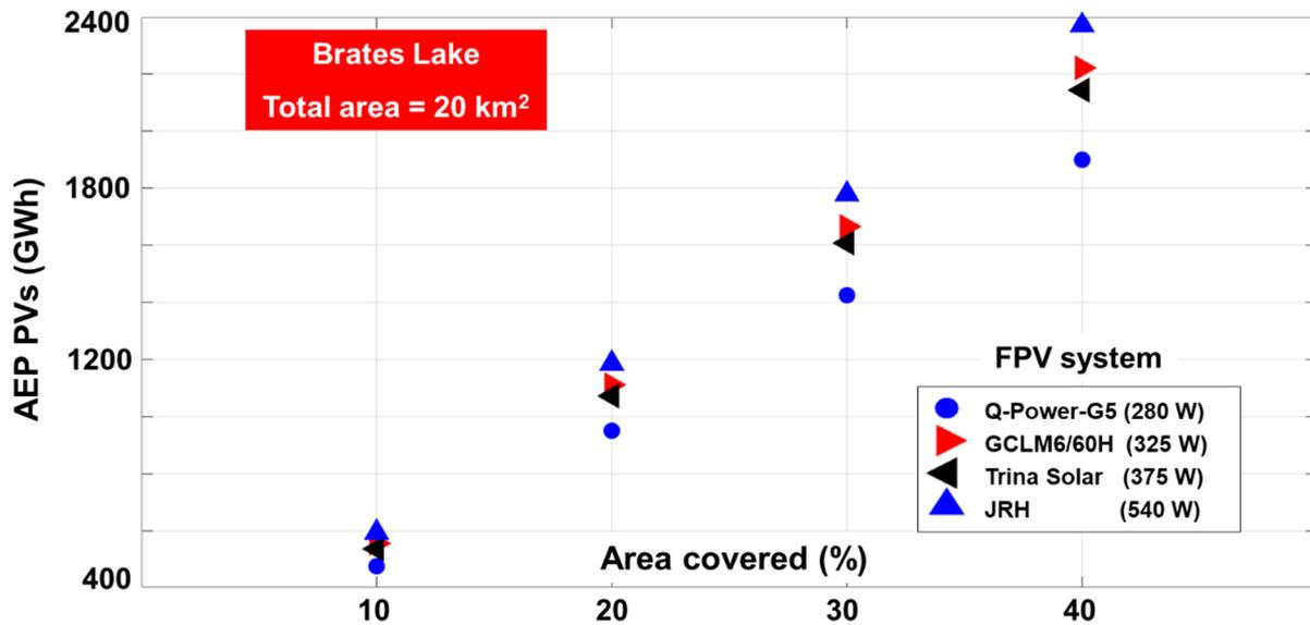
Figure 13. AEP performance of different floating PV modules operating on the Brates Lake. The results are based on ERA5 data (2001–2022), where the lake surface considered gradually increased from 10% to 40%, respectively.
