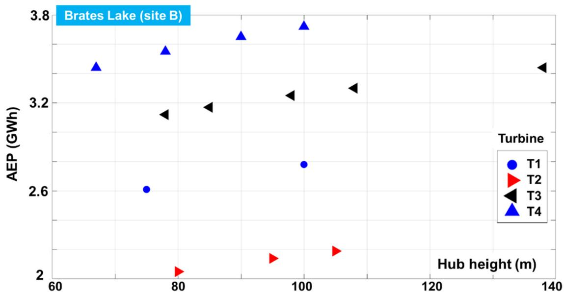
Figure 11. Brates Lake—AEP performance of the wind turbine considered, based on the ERA5 data (for the time interval 2001–2022). Results are processed for different hub heights.
