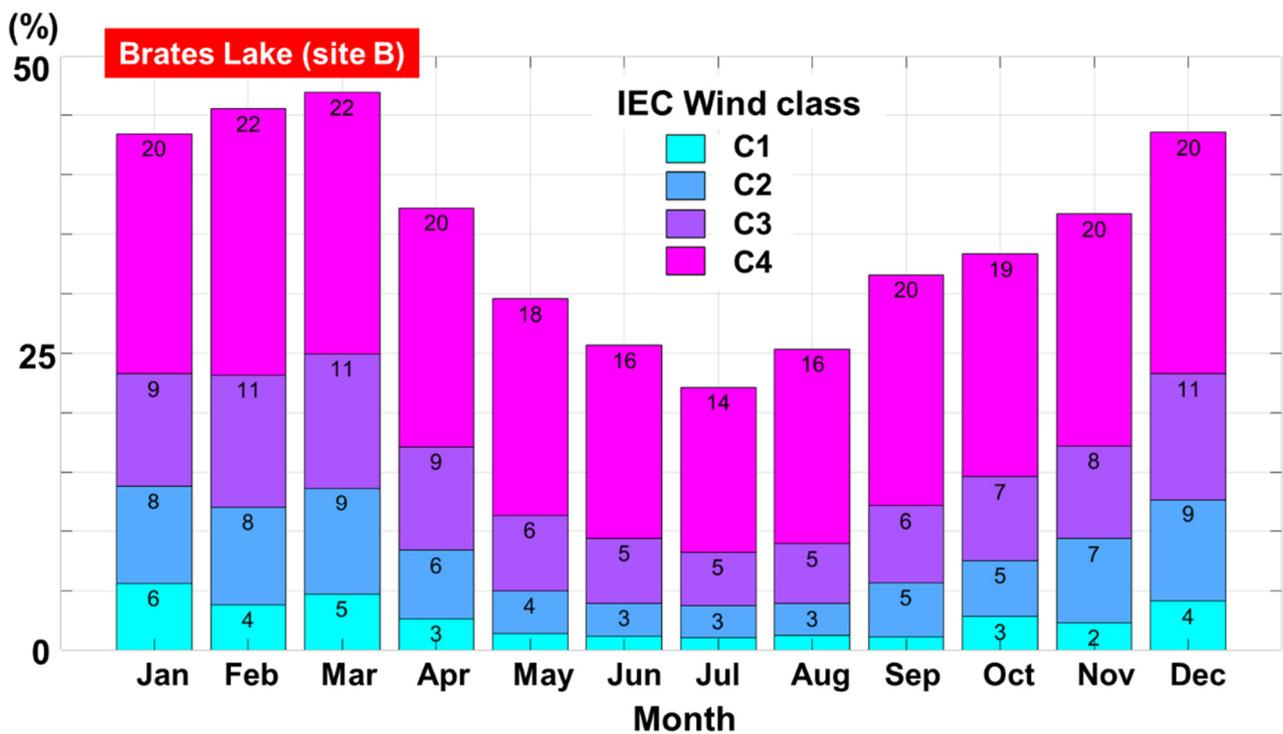
Figure 8. Monthly distribution of the IEC wind classes (ERA5 data) associated with site B. The results are defined for the interval 2001–2022, with a hub height of 100 m.
