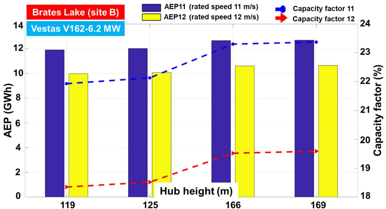
**Figure 12.** Performance of the Vestas V162-6.2 MW system expected from the Brates Lake location, according to the ERA5 data (for the time interval 2001–2022). The AEP and capacity factor are estimated for different hub heights and rated wind speeds (11 m/s and 12 m/s) of this generator.
