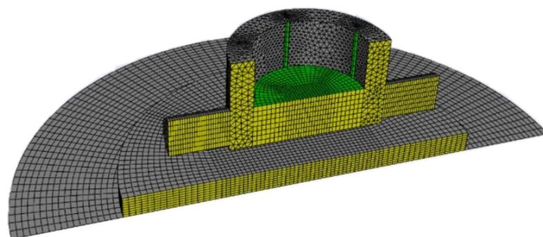
**Figure 10.** Ansys Fluent dynamic zone mesh preview using default colours. Yellow regions indicate some parts of critical dynamic meshing, and green region indicate an example of the consequence influence of the dynamic region.
