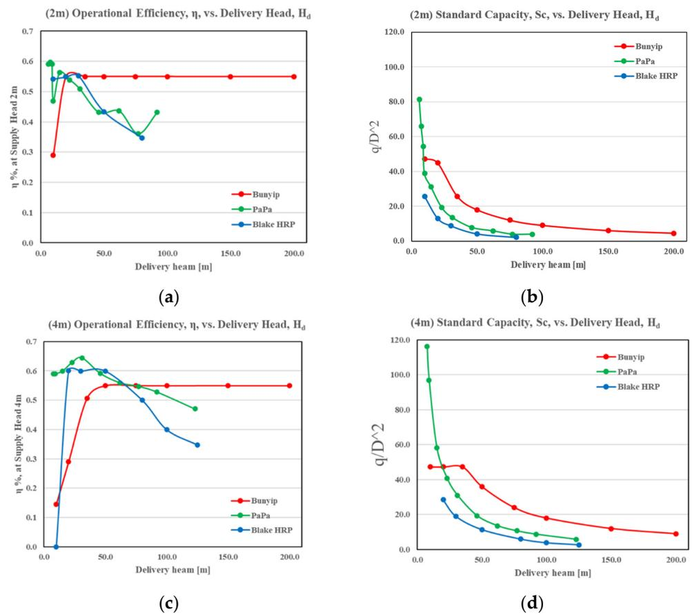
**Figure 5.** Graphical performance evaluation at 60 L/min and 2–4 m supply heads for the 3 pump systems (a) efficiency at 2 m supply head, (b)  $S_c$  at 2 m supply head, (c) efficiency at 4 m supply head, and (d)  $S_c$  at 4 m supply head.
