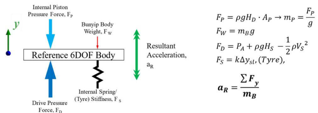
Figure 11. Free-body diagram and determination of 6DOF solver’s properties.
