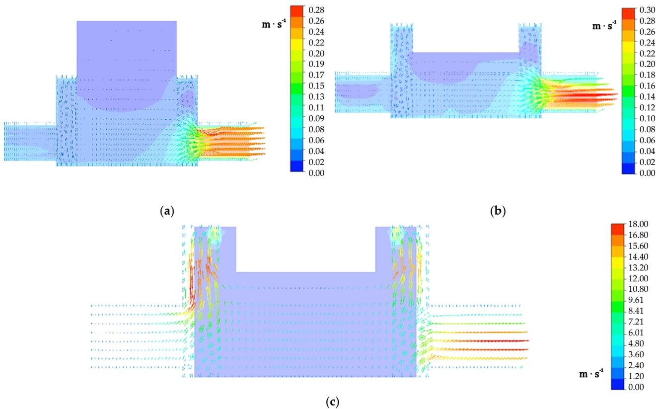
**Figure 16.** Velocity contours in the upper piston stroke and discharge regions, illustrating the transient motion vectors at different time instants for (a) delivery stroke at 0.1 s; (b) water delivery as piston approaches BDC of the power stroke at 1.875 s; and (c) waterflow accelerates from the domain to the three exhaust points at 1.91 s.
