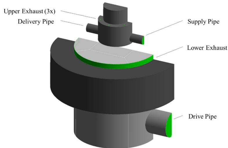
**Figure 12.** Annotated Bunyip pump for boundary condition definition.
