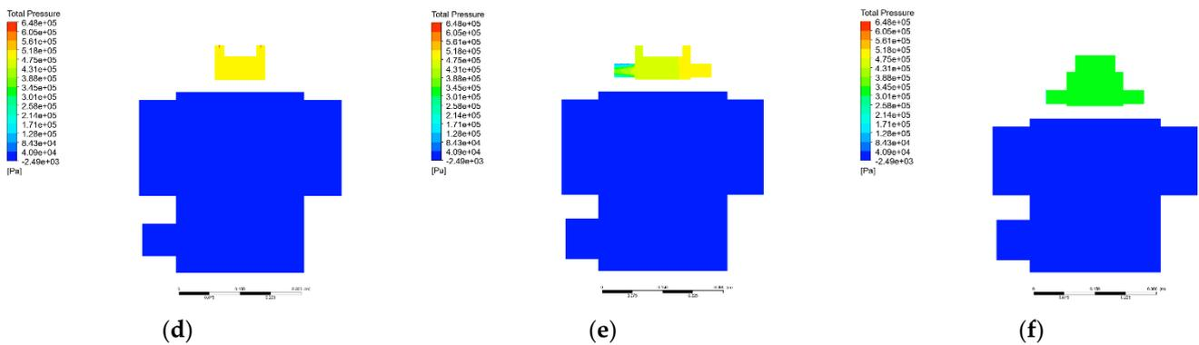
**Figure 13.** Illustration of Bunyip cycle’s internal total pressure distribution. (a) At 0.1 s: delivery stroke start; (b) 1.0 s: mid-delivery stroke; (c) 1.875 s: piston approaches BDC; (d) 1.925 s: upper piston discharge ‘Un-lock’; (e) 2.025 s: piston prime initiates using supply; (f) 2.4 s: operational cycle complete.
