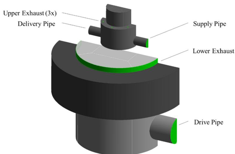
**Figure 12.** Annotated Bunyip pump for boundary condition definition.
