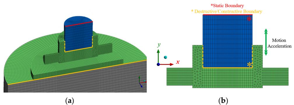
**Figure 9.** Dynamic mesh zone setup, showing (a) isometric and (b) front cross-sectional views. Green regions depict rigid body motion, blue depicts active dynamic layering in the upper piston, and grey depicts the interface between the static tyre/base.
