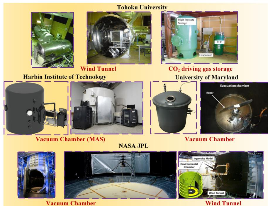
Figure 7. Mars atmospheric environment simulation setups.
