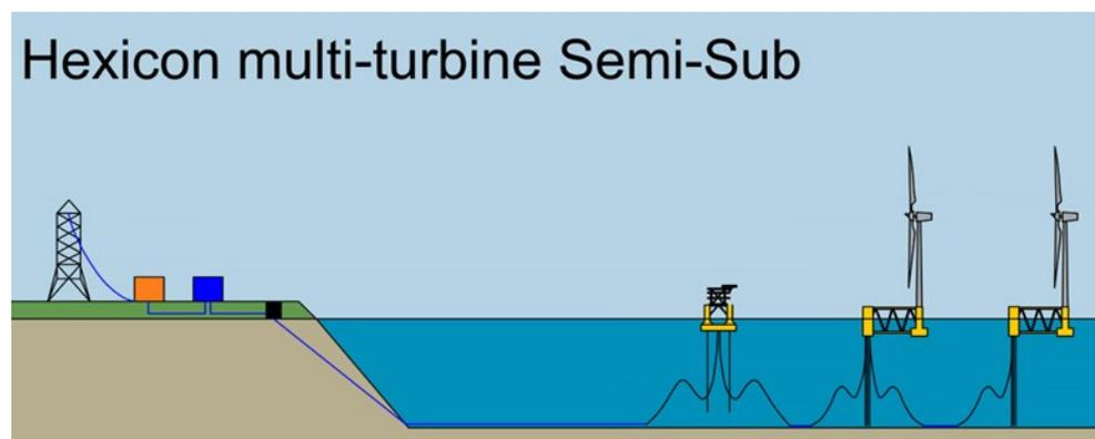
**Figure 6.** The most widely used multi-turbine floating wind turbine support structure in the world (HEXICON). Figure processed by the authors on the basis of information presented in [78].
