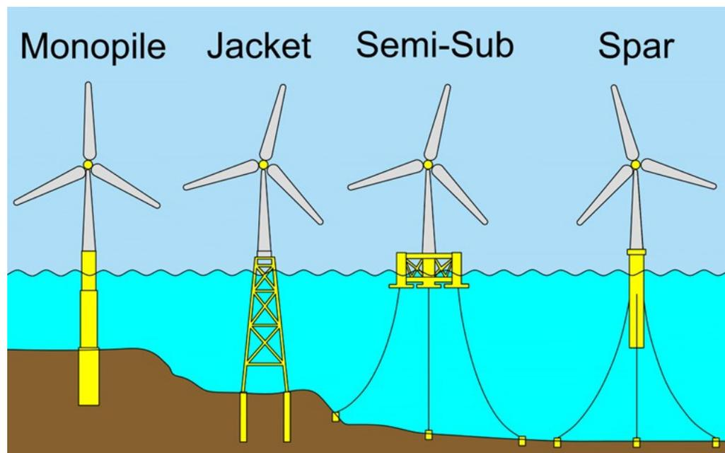
**Figure 1.** Most widely used bottom-fixed and floating wind support structures in the world, indicated. From left to right: monopile, jacket, semi-submersible, and spar-buoy. The authors processed the figure in accordance with the information presented in [10].
