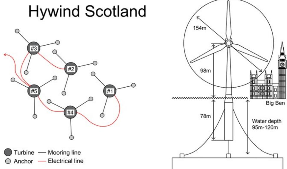
**Figure 5.** The first installed floating wind project in the world (Hywind Scotland). Figure processed by the authors on the basis of information presented in [77].
