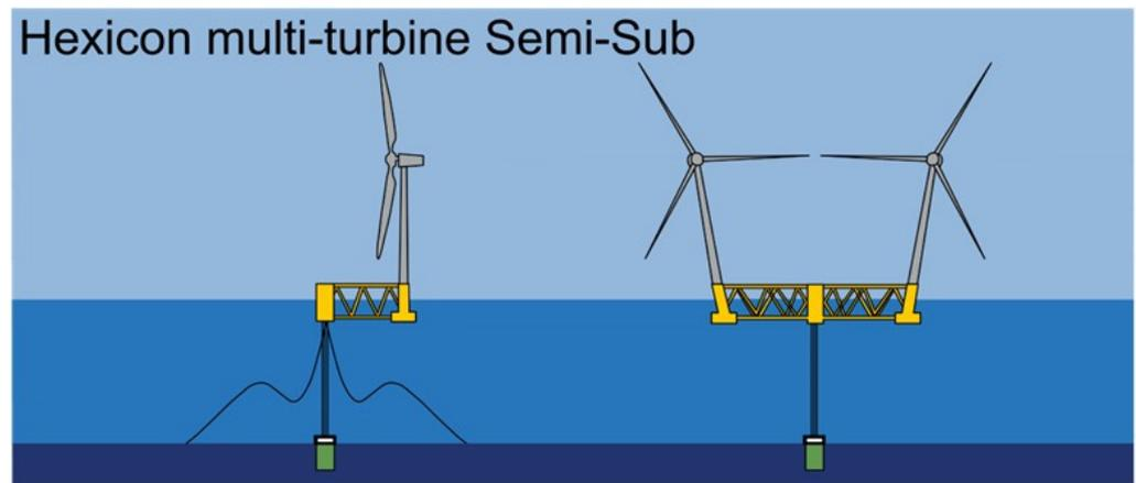
**Figure 7.** The most widely used multi-turbine floating wind support structure in the world (HEXICON). Figure processed by the authors on the basis of information presented in [78].
