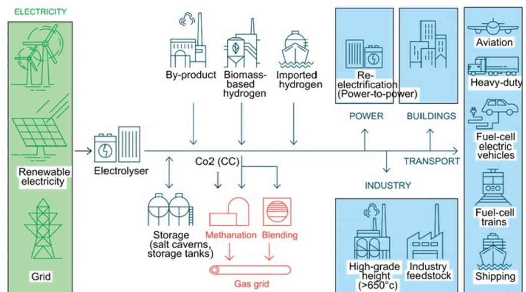
**Figure 9.** The floating wind Power-to-X technology, that transforms the produced floating wind electrical power (mainly into hydrogen and compressed air). Figure processed by the authors on the basis of information presented in [79].
