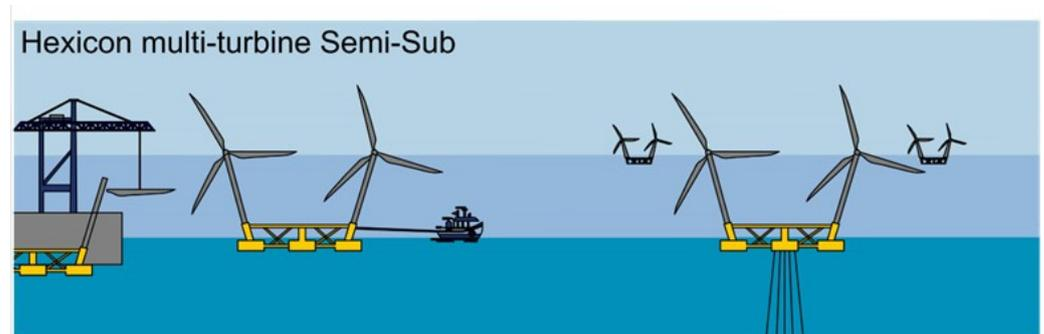
**Figure 8.** The most widely used multi-turbine floating wind support structure in the world (HEXICON). Figure processed by the authors on the basis of information presented in [78].
