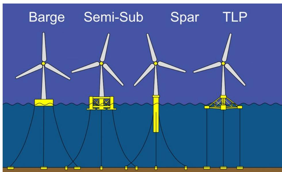
**Figure 2.** Most popular floating wind support structures in the world. From left to right: barge, semi-submersible, spar-buoy, and TLP. Figure processed by the authors according to the information presented in [10].
