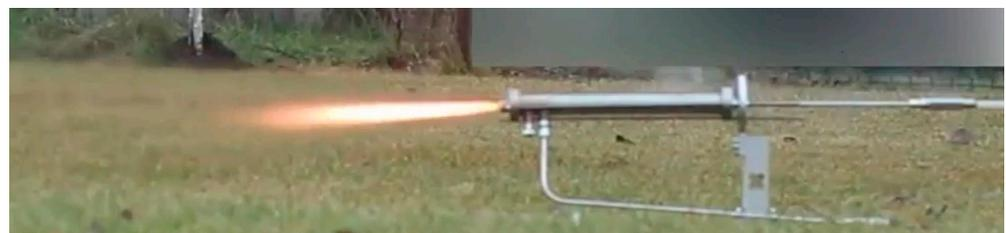
**Figure 22.** Hybrid rocket motor during functioning.
