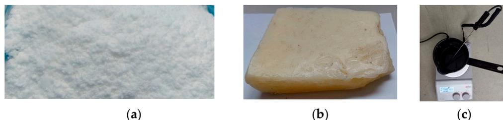
**Figure 3.** Preparation of paraffin and paraffin mixture: (a) paraffin wax solid grain, (b) prepared paraffin wax, and (c) heating at 76.8°C and mixing the paraffin and new propellant.
