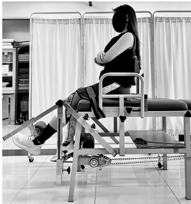
Figure 1. Maximum voluntary contractions (MVCs) test using the push–pull dynamometer that was mounted to the NK table’s leg.
