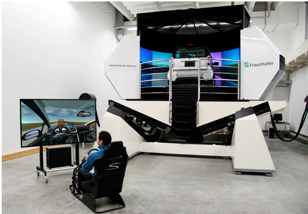
Figure 1. Platform for networked driving simulation at the University of Paderborn in Germany.
