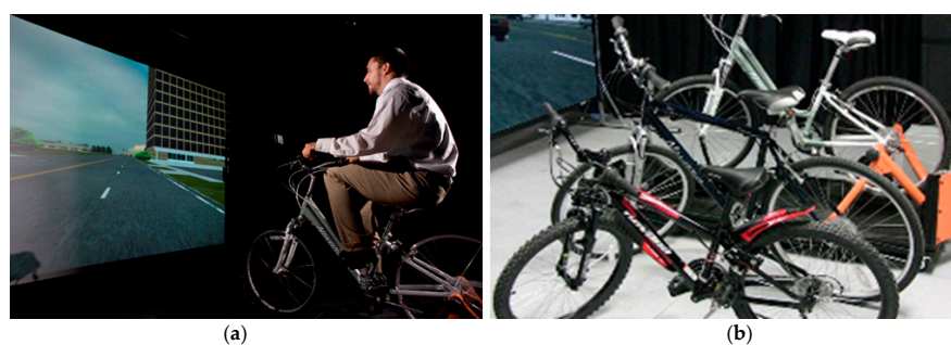
Figure 9. Bicycling simulator at the Oregon State University (OSU): (a) A test person riding the bicycle simulator; (b) Different bicycle variants [43].
