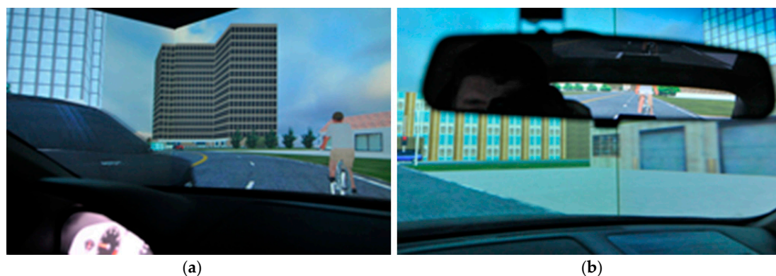
Figure 10. Two different virtual scenarios combining a vehicle and a bicycle controlled by humans (OSU): (a) A vehicle behind a bicycle; (b) A bicycle behind a vehicle [43,44].
