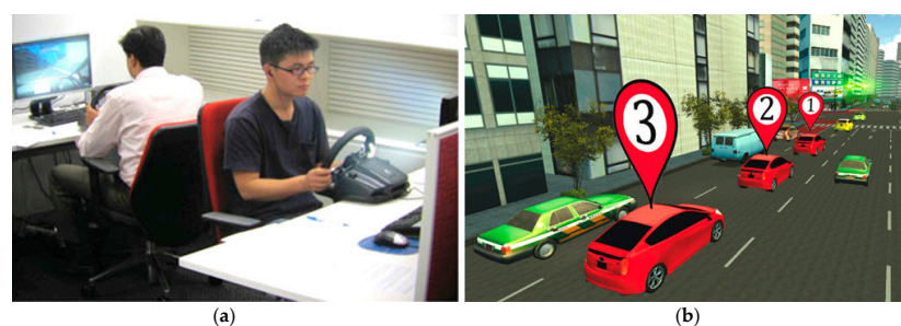
Figure 7. Tokyo Virtual Living Simulation Lab at NII: (a) Test persons using two networked driving simulators; (b) A screen shot of a shared 3D environment [41].
