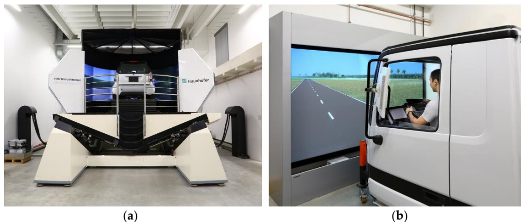
Figure 1. Two driving simulator variants at the Heinz Nixdorf Institute in Germany: (a) Passenger car driving simulator with a motion platform; (b) Stationary truck driving simulator.
