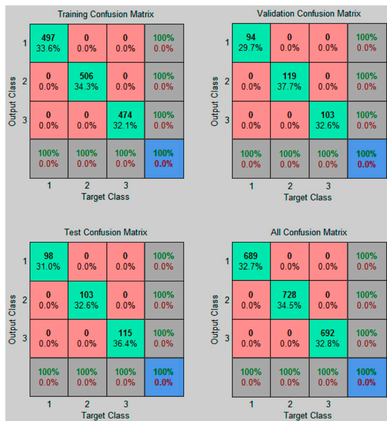
Figure 11. Confusion matrix resulted after training process where 100% of data is classified correctly.
